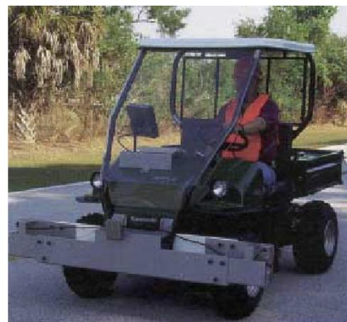
**Abbildung 2-19: Dual Track Profiler ICC [17].**
