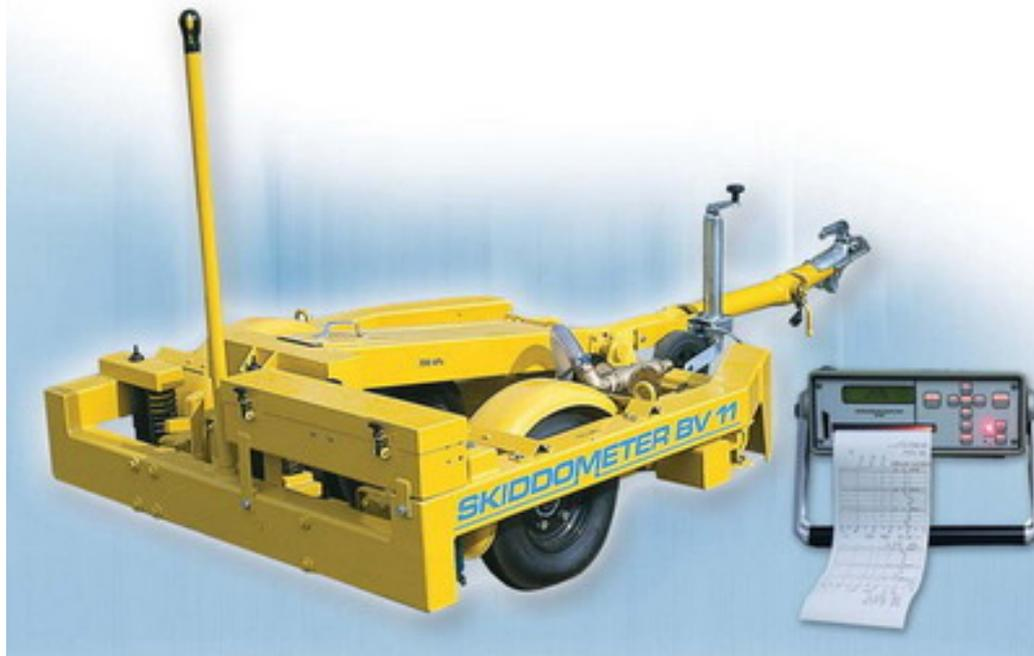
Abbildung 3-36: Skiddometer Trailer [71]
