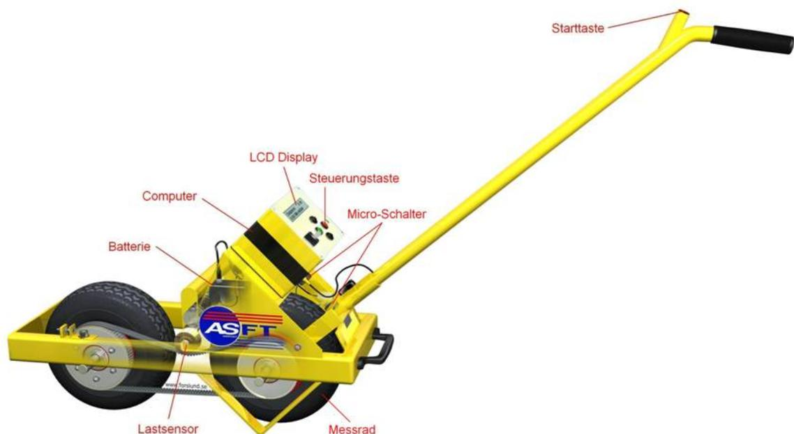
**Abbildung 3-38:** T2GO Portable Friction Tester [74]
