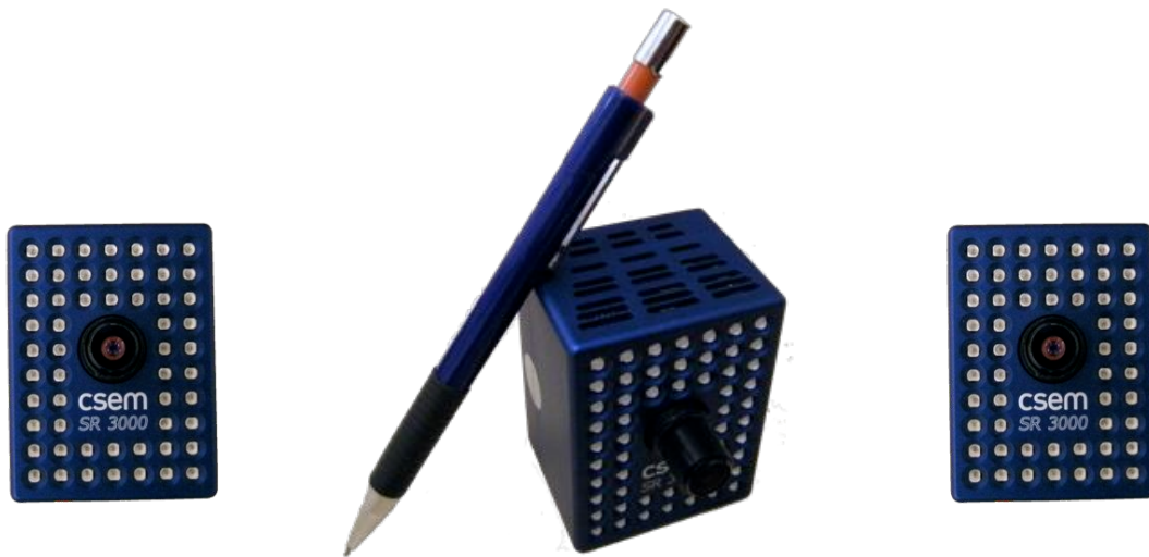
Figure 3.1: Front pictures of SR3000. LEDs are placed around the mounted optical lens. Slots on the top provide a cooling facility.
