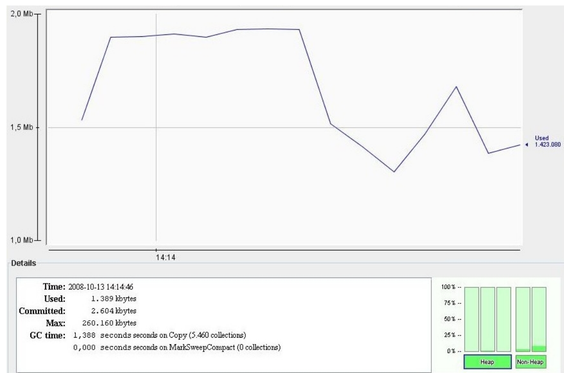
Figure 5.8: Heap space consumption on 250k rows WebRowSet with the novel implementation
