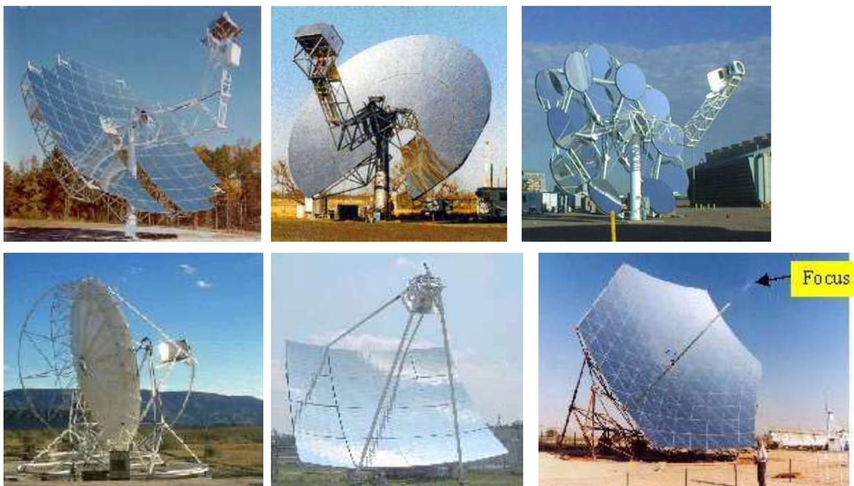
Figure 3.15 Six different dish systems: McDonnell-Douglas (upper left), WGAssociates (upper middle), SAIC (upper right), Schlaich Bergermann und Partner (bottom left), HiTek's 14 m<sup>2</sup> dish prototype (bottom middle) and the Australia National University 400 m<sup>2</sup> dish
