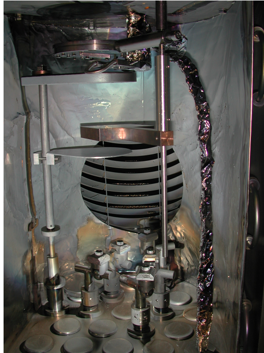
Figure 5.4: Modified sample holder in the evaporation device. The original one is the surface located in the upper area, the new one is that in the central area.
