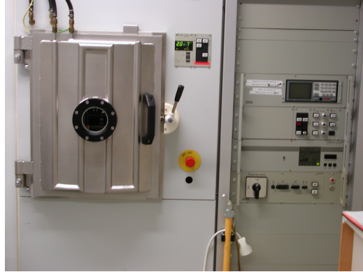
Figure 5.3: Balzers evaporation device: The evaporation process is started at a pressure of 10^{-6} mbar. The current for the evaporation is controlled by a potentiometer at the control panel. The indicator for the deposition rate also situated there has to be calibrated by a factor of 7, because the sample holder is mounted nearer to the evaporation source than that for usual samples.
