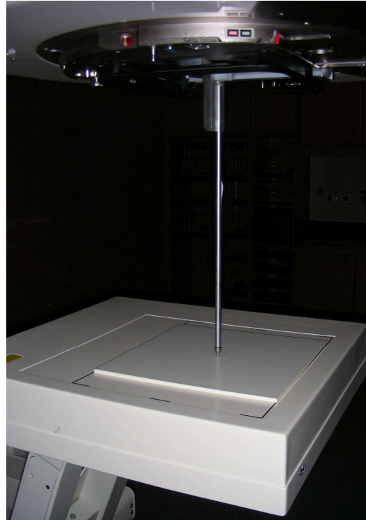
FIG. 47, RW3-slabs on top of the EPID
