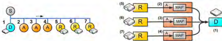
Figure 5.5: CashFlow Scene Graph Example with several MultiData nodes (left): One MultiData(D), three DataAccess(A) and a Render(R) node. Process flow (right): Each Render node [5][6][7] links to a separate DataAccess node [2][3][4] and accesses the DataAccess map(grey) inside. All DataAccess map's (grey) refer to the same MultiData nodes [1]. Although this process flow differs from figure 5.3 and figure 5.4 the visual result may stay the same.
