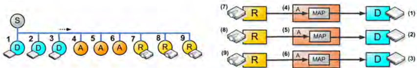
Figure 5.6: CashFlow Scene Graph Example with several MultiData nodes (left): Three MultiData(D), three DataAccess(A) and a Render(R) node. Process flow (right): Each Render node [7][8][9] is bound to a separate DataAccess node [4][5][6] using the embedded DataAccess map(grey). Each DataAccess map(grey) refers to a separate MultiData nodes [1][2][3]. Although the four introduced scene graphs look quite different, they may produce the same visual results, because of the DataAccess node interface.
