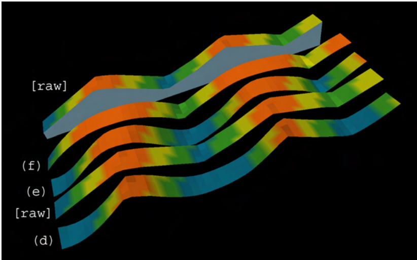
Figure 5.21: CashFlow Constant, linear and cubic parameterization: A color map was created for each height field. Letters indicate corresponding data sets in this figure and figure 5.20. The color map in this figure is bound to the actual height. This image also shows that the surrounding grey box can be disabled.
