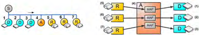
Figure 5.4: CashFlow Scene Graph Example with several DataAccess nodes (left): Three MultiData(D), one DataAccess(A) and a Render(R) node. Process flow (right): Each Render node [5][6][7] uses its own DataAccess map(grey) inside one DataAccess node [4] referring to several MultiData nodes [1][2][3]. This scene graph may produce the same output as scene graph from figure 5.3.
