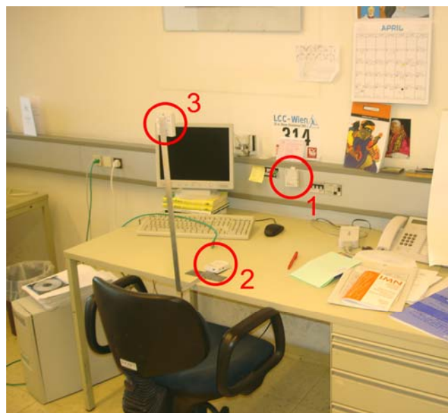
Figure 115. Equipment configuration for measuring illuminance for different positions - original (1), horizontal (2) and head (3) position
