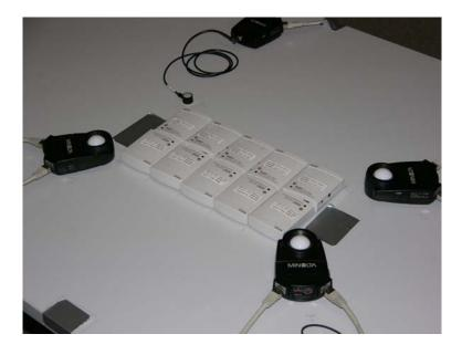
Figure 2-18 process to find the accuracy factor of the light sensors
