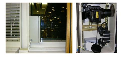
*Figure 2-11 Camera box with power supply pointing to the VC\_NO façade*
