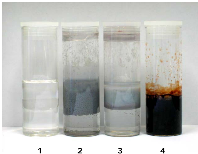
Figure 2.2. The four stages of silver nanoparticle synthesis: (1) TOABr in toluene over silver nitrate in water. Both phases are clear. (2) When the two-phase system is stirred, a white precipitate of AgBr is formed (very light sensitive, turns grey), which slowly transfers to the organic phase. (3) No change upon addition of dodecanethiol. (4) After addition of aqueous NaBH 4 solution, the organic phase turns brown, indicating the formation of silver nanoparticles.
