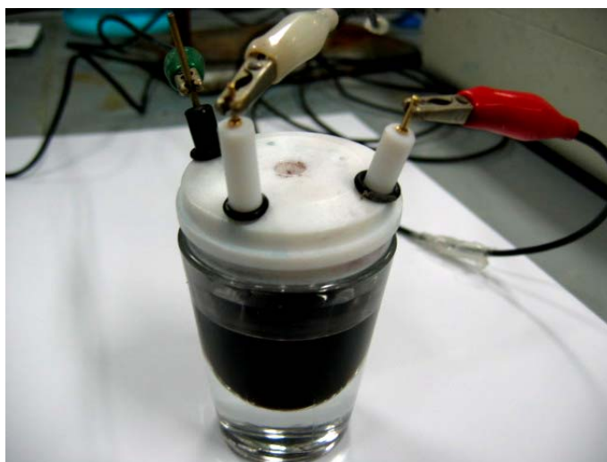
Figure 2.4. The electrochemical cell. Left: working electrode (green clamp), centre: reference electrode (white clamp), right: counter electrode (red clamp).
