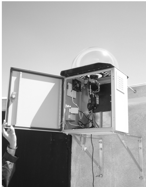
Figure 6.3: Sky-scanning camera mounted on main building roof.
