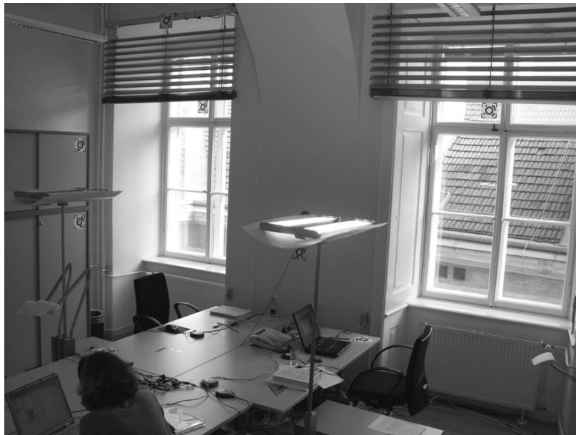
Figure 6.4: Test space with uplights and window blinds.
