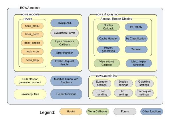
Figure 3: The main components of the EOWA module
