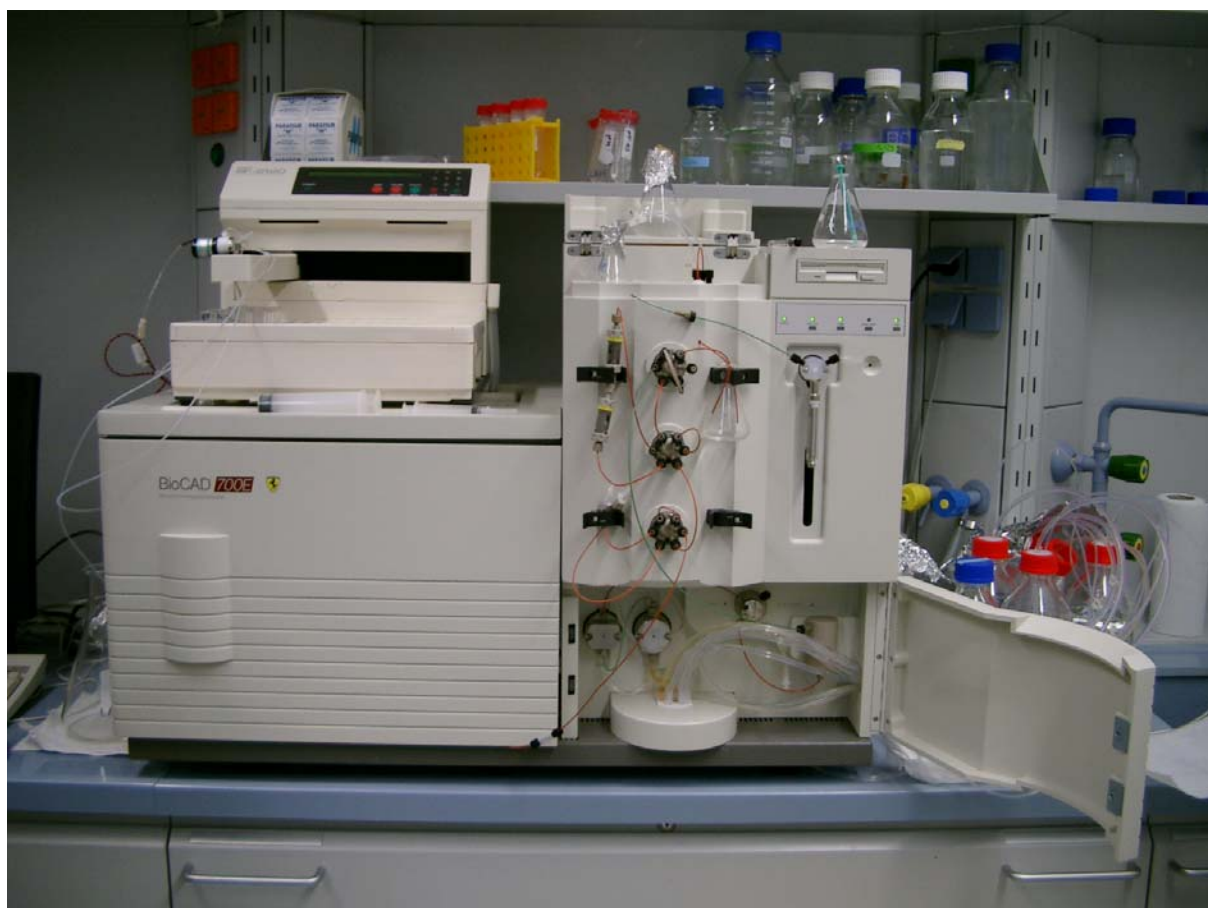
Fig. 20. The BioCAD 700E work station in process with two coupled POROS ® affinity depletion columns. The two columns, with a yellow mark, are visible in the center of the picture.
