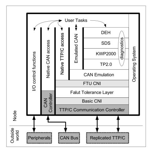
Figure 3.1: I/O interfaces of a node in our model and the associated layers
