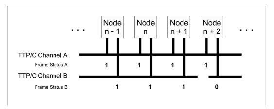
Figure 4.13: Frame statuses during simulated cable break
