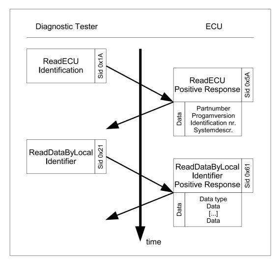
Figure 3.7: KWP2000 flow diagram
