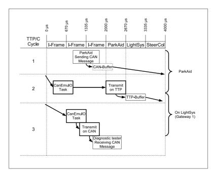
Figure 5.12: Latency: Parking Aid to Tester (Best Case)
