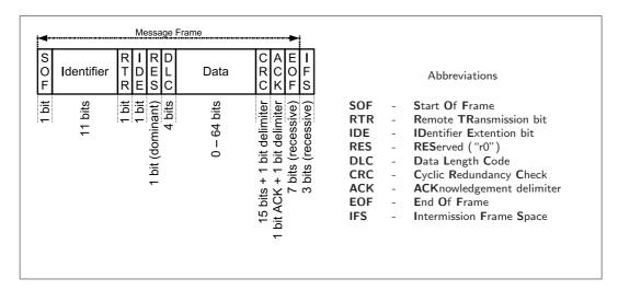
Figure 3.3: The standard CAN-Message Frame
