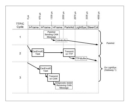
Figure 5.13: Latency: Parking Aid to Tester (Worst Case)
