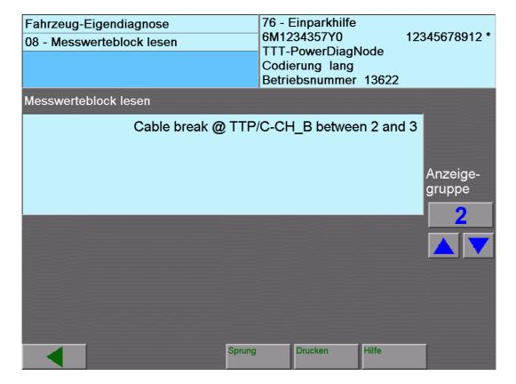
Figure 4.15: Sample diagnostic tester output during cable break
