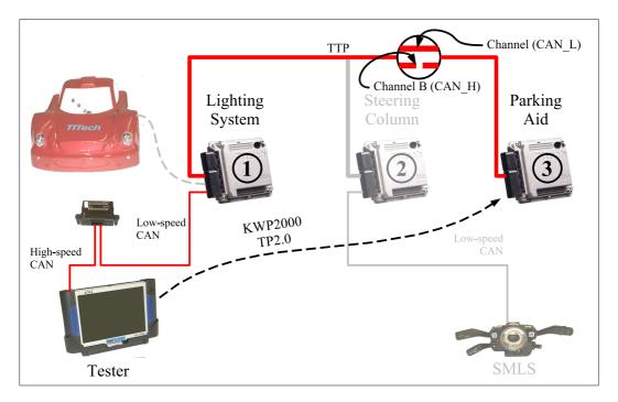
Figure 5.5: Cable break diagnosis using legacy tester hardware
