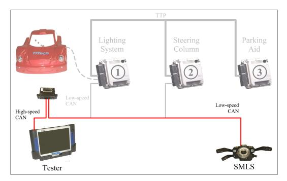
Figure 5.1: Standard CAN communication
