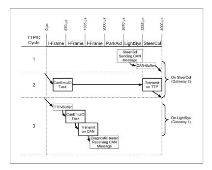
Figure 5.8: Latency: Steering Column to Tester (Best Case)
