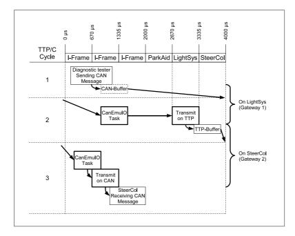
Figure 5.7: Latency: Tester to Steering Column (Worst Case)
