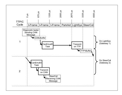
Figure 5.6: Latency: Tester to Steering Column (Best Case)
