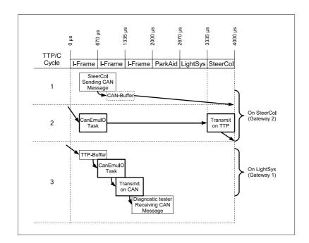
Figure 5.9: Latency: Steering Column to Tester (Worst Case)
