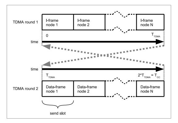
Figure 2.1: A cluster cycle with N nodes and two TDMA rounds
