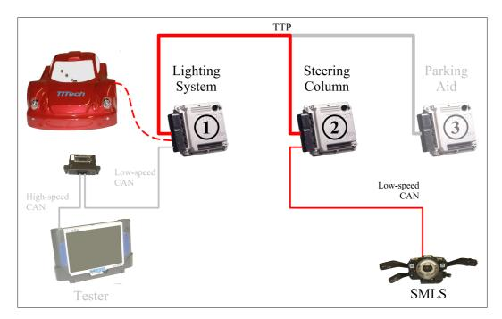
Figure 5.2: Controlling a TTP ECU with a legacy CAN ECU
