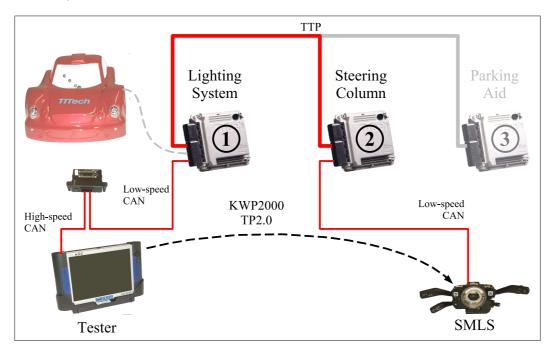
Figure 5.3: Tunneling CAN messages and diagnostic messages
