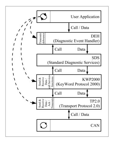
Figure 4.1: Call graph of the demo application provided by Audi.
