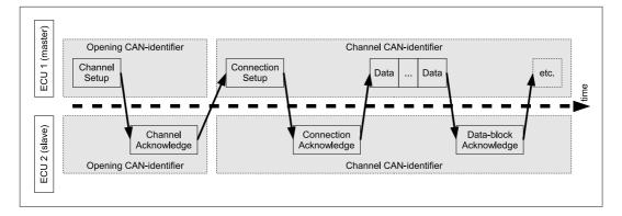
Figure 3.6: TP2.0 - Dynamic Channel Setup
