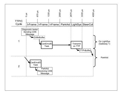
Figure 5.10: Latency: Tester to Parking Aid (Best Case)
