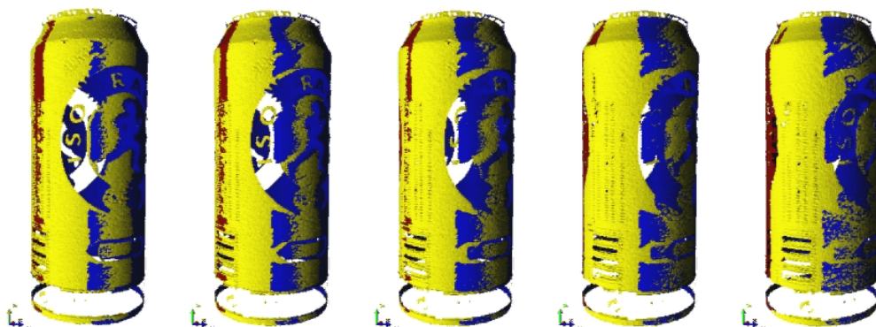
Figure 2.1: Tangential movement on rotational symmetric surface (Positions shown for iteration 1, 9, 17, 25, and 33 from left to right. The yellow point set can be seen to slide on the others, note the barcode field.)
