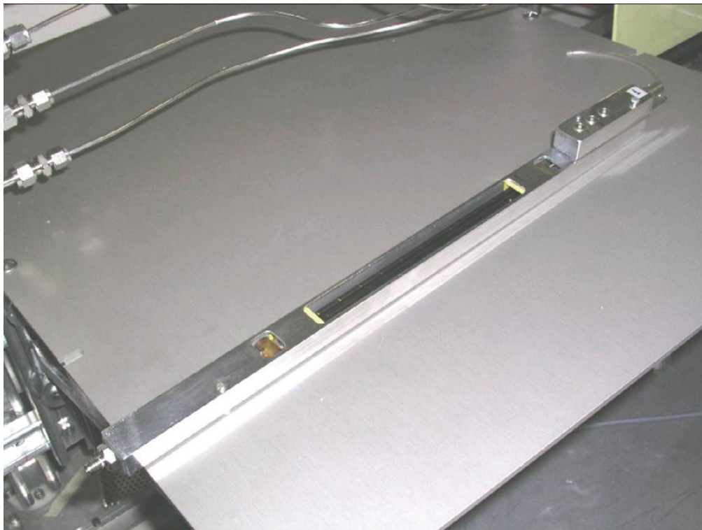
Figure 74: Straw prototype with three TRT straws connected in parallel
