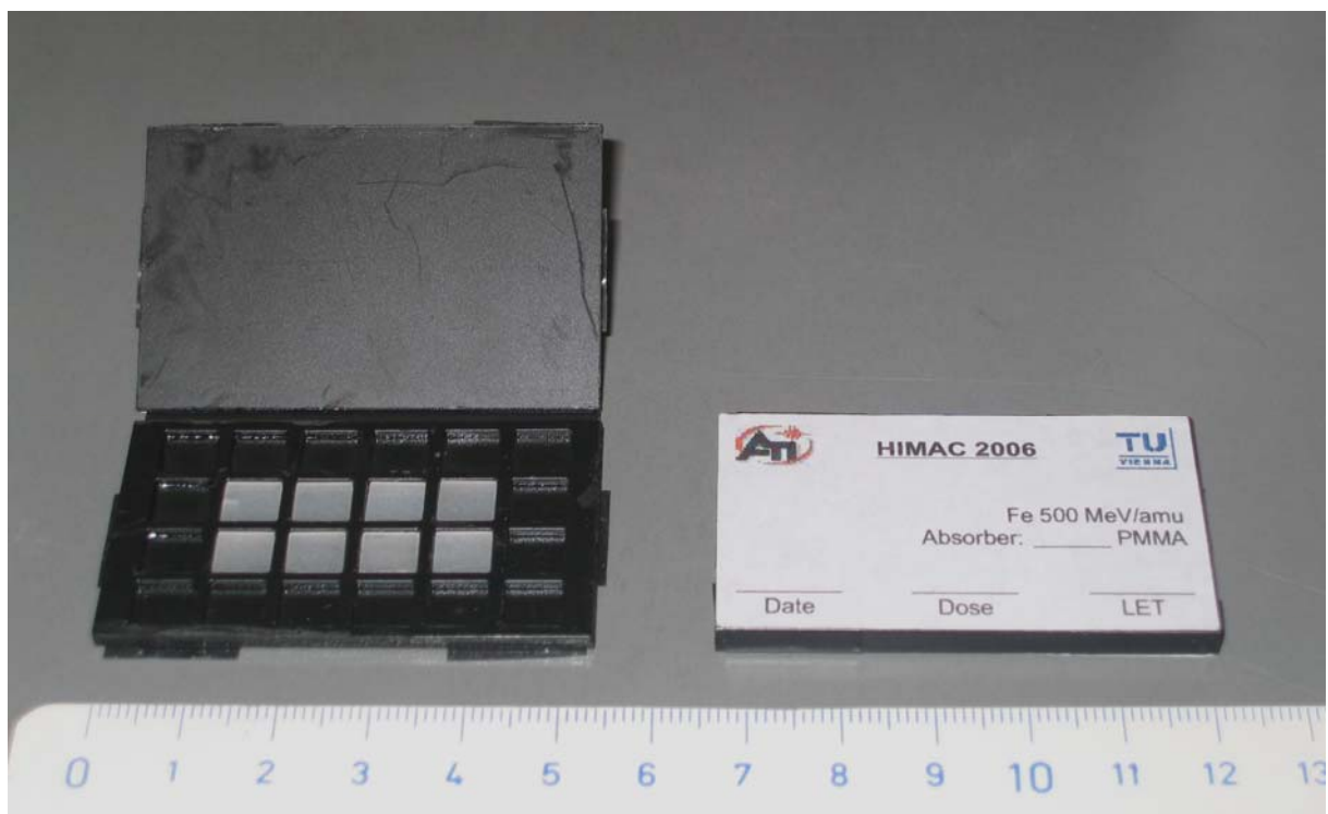
Figure 7.3. Two packages of TL dosimeters. 4 TLD-600 (upper row) and 4 TLD-700 (lower row) detectors in a polystyrene matrix (left) and an identical, closed and sealed package labelled for exposure at the HIMAC facility (right). A cm-scale is viewed as size reference.
