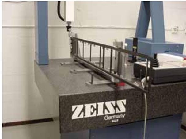
FIGURE 10.17: Rod frame measured by a CMM.
