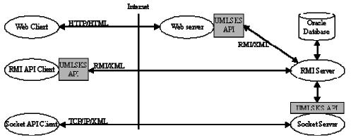
Figure 2-7 Diagram of the logical Architecture UMLSKS [14].
