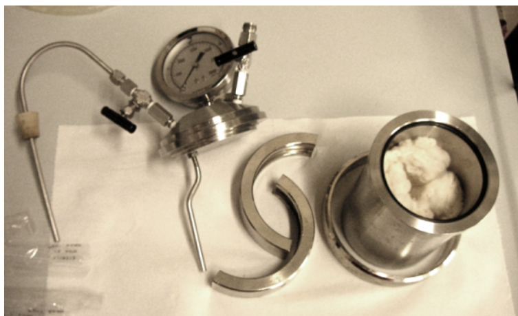
Figure 5.2: To the right the container for nitrogen pressurization of the algae can be seen (also called a "Nitrogen-bomb"). The top piece as seen in the left part of the image accommodates a pressure gauge and two valves to pressurize the container and to rapidly depressurize it.
