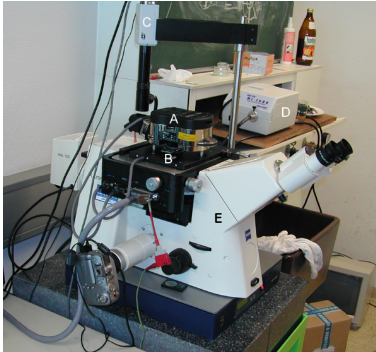
Figure 5.4: The AFM setup at the Institut für Allgemeine Physik at the TU Vienna. A - Scanning Head, B - Scanning Stage, C - Top View Optics, D - Top View Optics Light Source, E - Zeiss Inverted Optical Microscope
