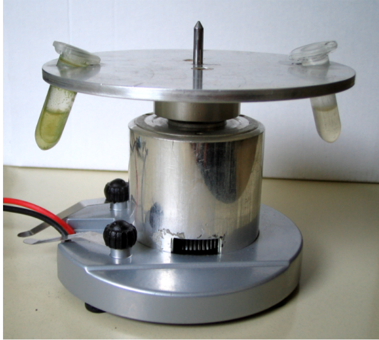
Figure 5.8: A small centrifuge was built (with the help of the supportive staff of the mechanical workshop at the TU-Wien) for the condensing of cell parts in the solution for the AFM. Here it is seen equipped with a vial of growth medium containing living algal cells (left) and a counterweight vial filled with water to the right.
