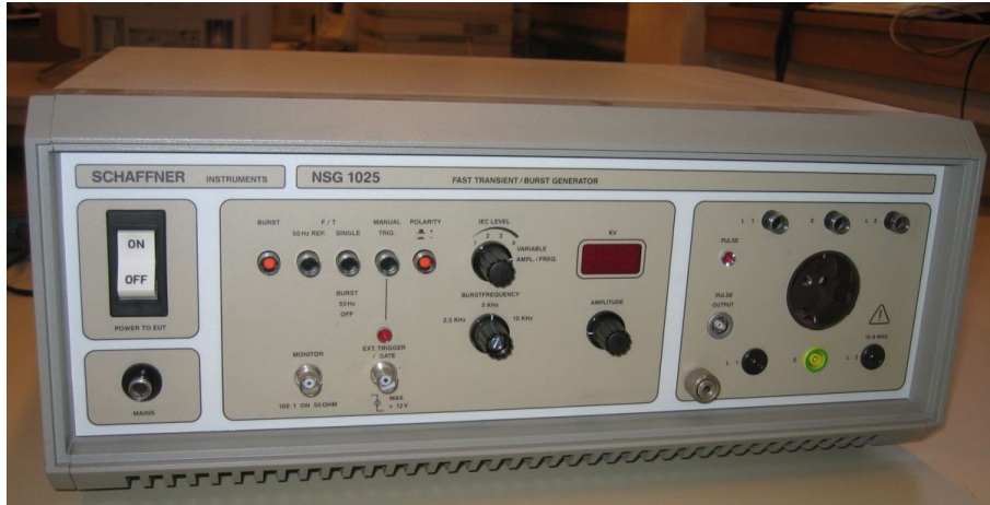
Figure 7.2: The NSG 1025 Fast Transient/Burst Generator
