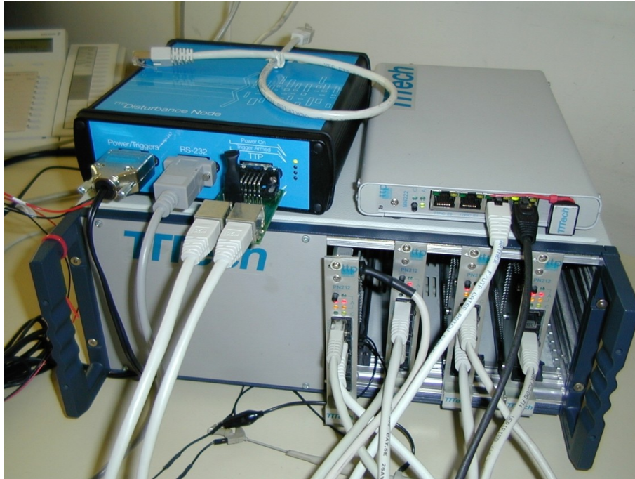
Figure 7.7: Fault Injection using the Disturbance Node
