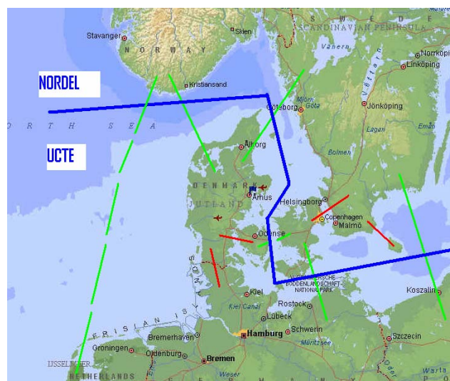
Figure 3.2 Border line between UCTE grid and Nordel grid, Showing DC connection lines crossing the border of the UCTE grid and the Nordel grid and AC connection lines within the systems, dotted lines are commissioned but not built yet; Source: (Togebly, M.; 2007)
