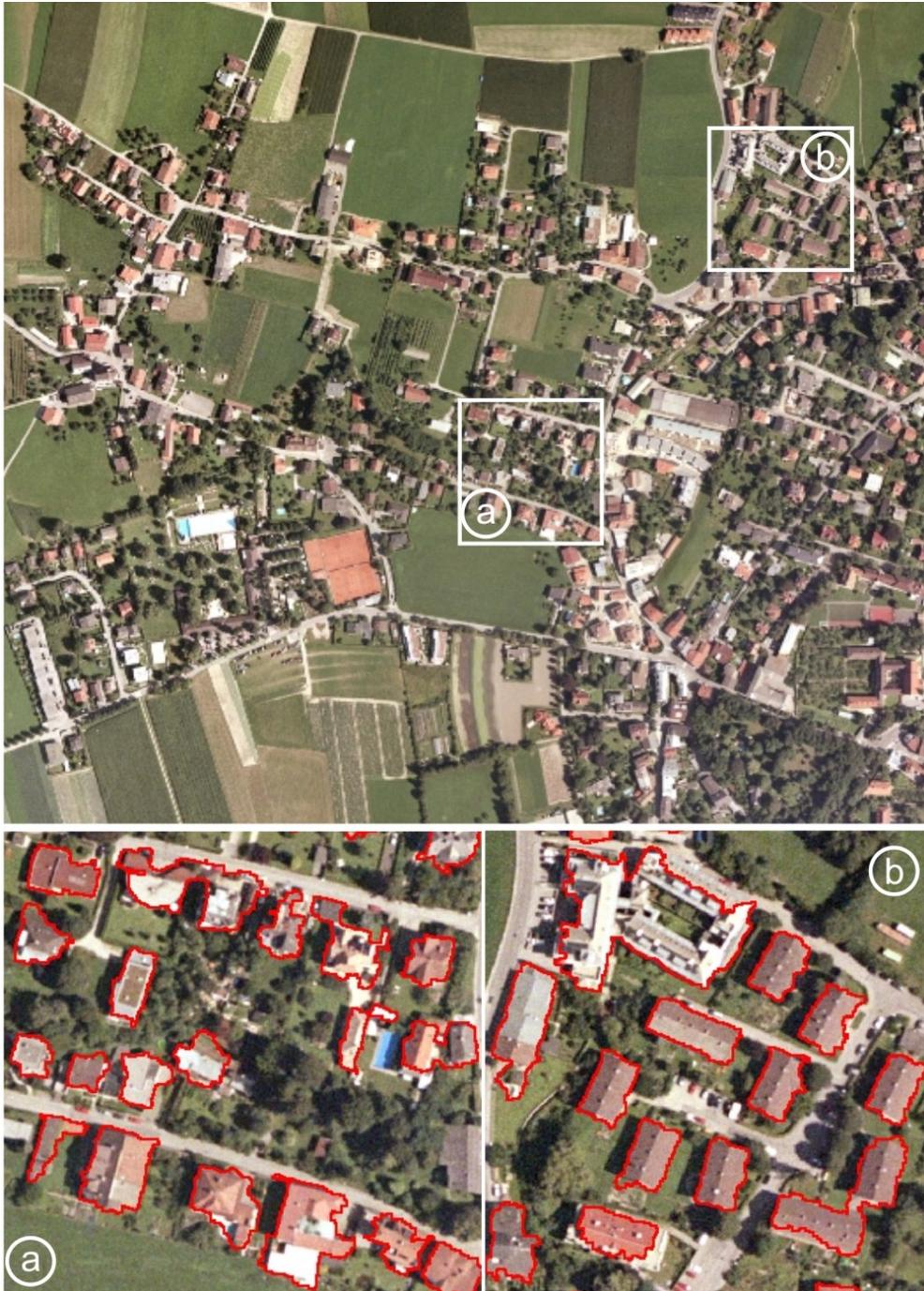
Figure 4.1: Test area Hall in Tirol. The ground resolution of the true-colored orthophoto is 0.25 m. In the more detailed figures a and b the building polygon data is added.
