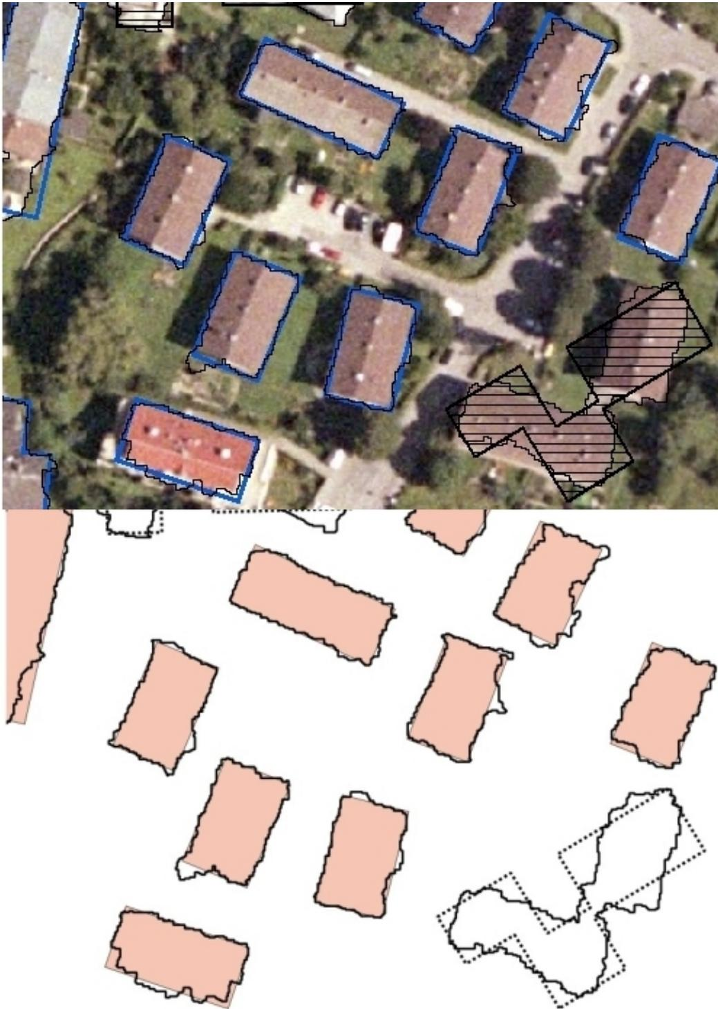
Figure 4.5: Detail of the generalization result with and without orthophoto. Blue polygons are valid generalizations, the ruled polygon has to be edited manually.
