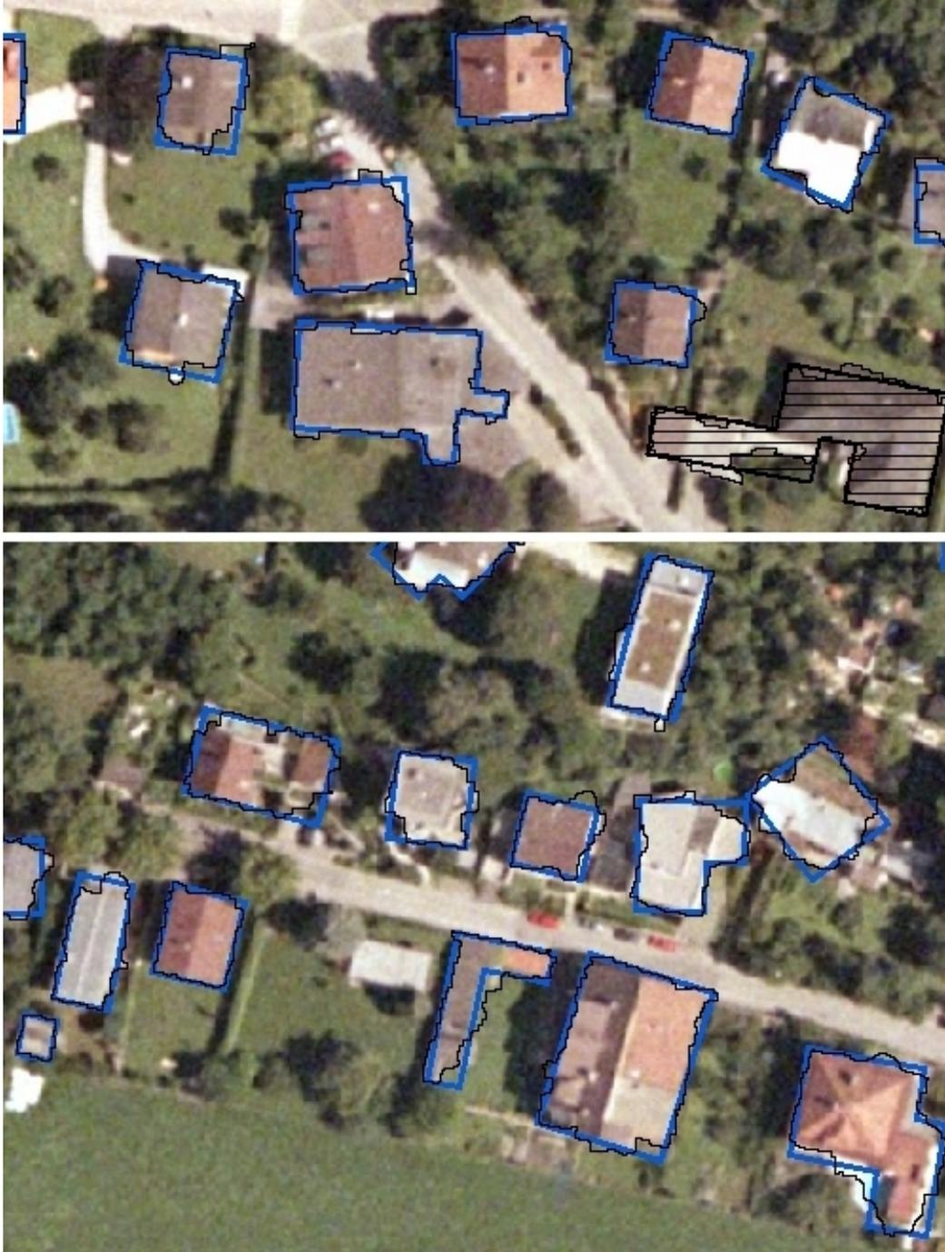
Figure 4.6: Detail of the generalization result. Blue polygons are valid generalization, the ruled polygon has to be edited manually.
