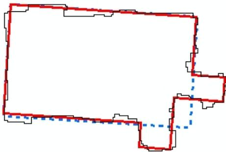
(a) Satisfying classification: Both generalized polygons are accepted by the tool. Red polygon:  $V=2.5\text{ m}$ ; blue, dashed polygon:  $V=3\text{ m}$
