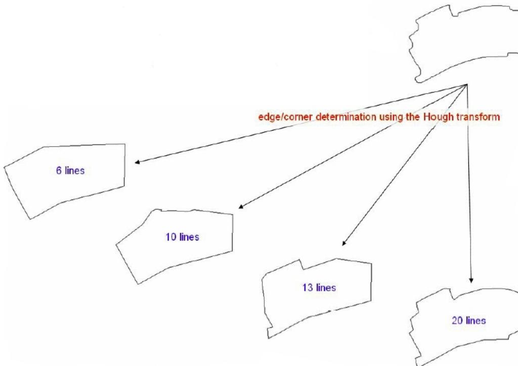
Figure 2.14: The level of detail can be controlled by the count of lines, thus the count of searched local maxima. From: (Vozikis 2005).
