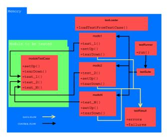
Figure 4: Unit Test Memory Layout (case 2)
