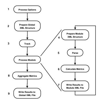
Figure 12: The Main Logic of the New Unit Test Framework
