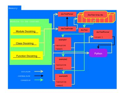
Figure 6: Docstring Test Memory Layout
