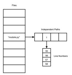
Figure 13: Tracks Data Structure
