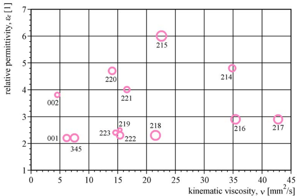
Fig. 6-44: Correlation between the sizes of damaged regions at bearing balls and the relative permittivities and kinematic viscosities of the oil samples (numbers according to Tab. 4-1) used for EDM-test series. The areas of the circles are proportional to the damaged regions (ellipses) at the surfaces of the bearing balls after approximately 16000 EDM-events at 80 °C. The mid points of the circles indicate the viscosities and relative permittivities of the oil samples at the respective temperature.
