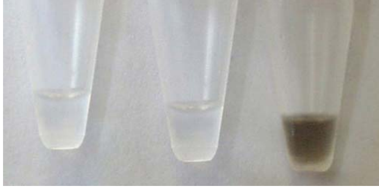
Fig. 6-15: Appearance of di-2-ethylhexyl-sebacat (002) unstressed (left), after 32000 EDM-events initiated in the static test rig with a voltage of 12 V (middle) and of 120 V (right).
