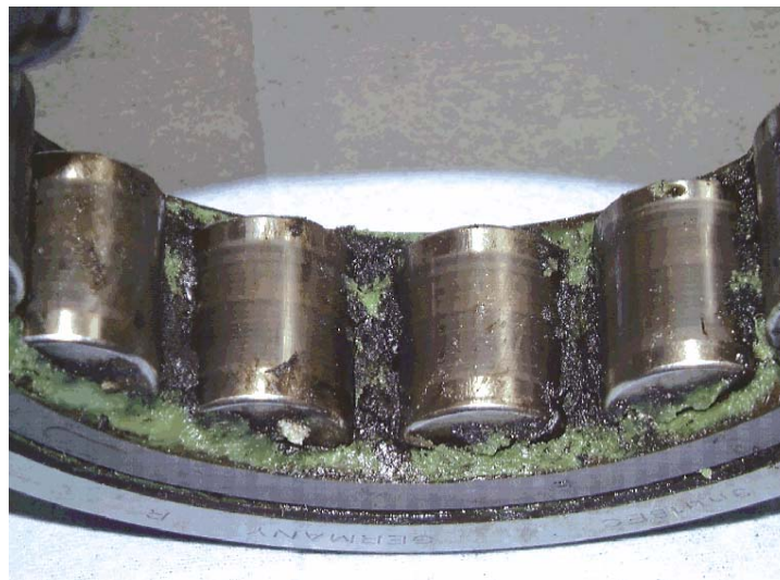
Fig. 2-7: Deterioration of a lubricant due to electric current passage [2]. Wide regions of the lubricant appear black discoloured by burned carbon deposits and lubricant caking.
