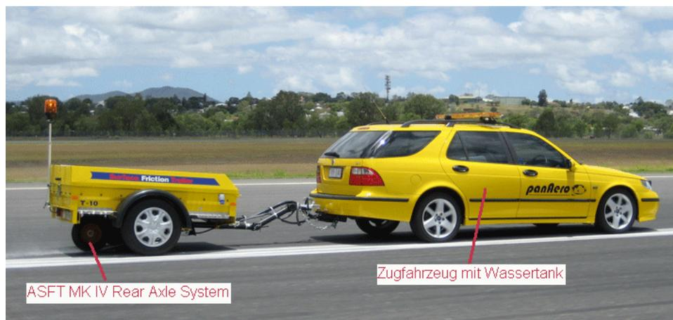
Abbildung 5-37: ASFT T-10 Trailer Road Friction Tester [ASFT, 2007].
