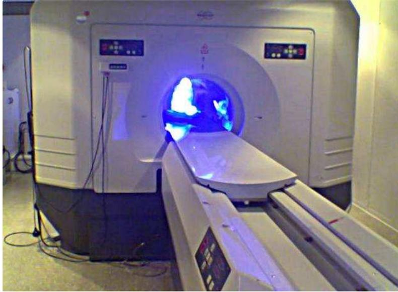
**Figure 3.1:** The 3 T Bruker Medspec S 300 DBX whole-body scanner (Bruker Biospin, Ettlingen, Germany), installed at the MR Centre of Excellence, Vienna Medical University. The inner diameter of the magnet bore including the whole-body gradient system is 55 cm. A background light is shining through a glass sphere.
