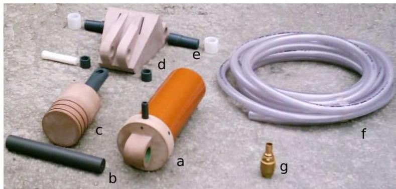
**Figure 3.3:** Individual parts of the ergometer's pneumatic system and pedal: cylinder (a) and its axis (b), piston (c), pedal (d) and its axis (e), flexible pneumatic tube (f), throttle valve (g) connecting tube and reservoir (not shown).
