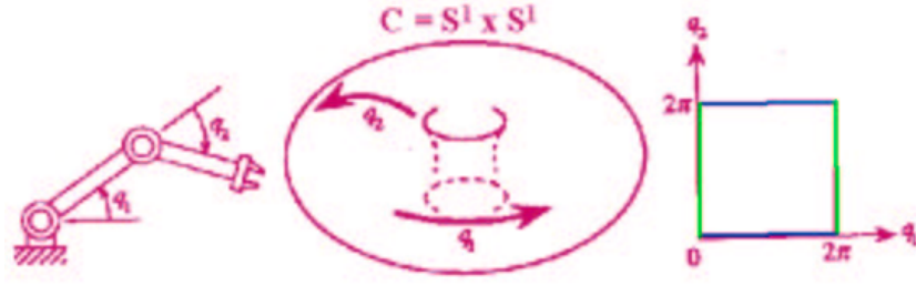
Fig. 3.4.: A 2 DOF Articulated Robot and it's configuration space
