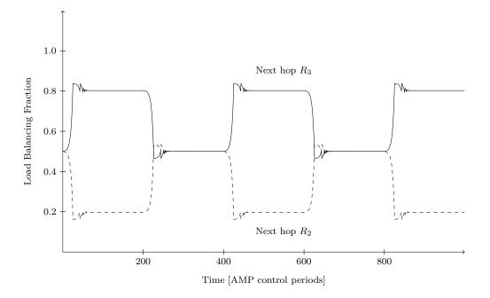
Figure 4.4.5: Load distribution in  $R_1$  in Experiment 2.
