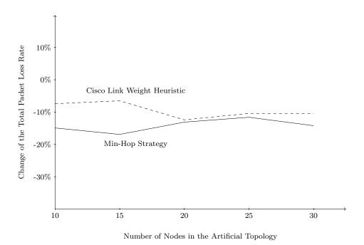
Figure 4.3.6: AMP in artificial topologies running CBR traffic with  $\alpha = 5\%$  and  $\beta = 125\%$ .
