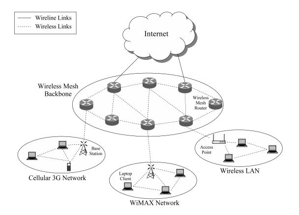
Figure 6.3.3: Example of a hybrid wireless mesh network.
