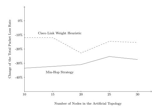
Figure 4.3.4: AMP in artificial topologies running CBR traffic with  $\alpha = 5\%$  and  $\beta = 115\%$ .
