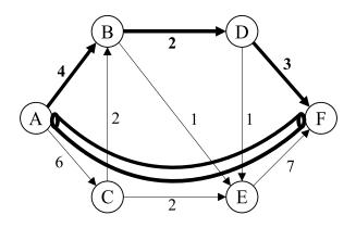
Figure 2.2.3: Arbitrary MPLS tunnel from node A to node F,  $A \to C \to E \to F$  which disregards the shortest path according to the link weights,  $A \to B \to D \to F$ .
