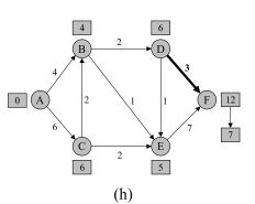
Figure 2.1.4: Illustration of the generic label correcting algorithm.
