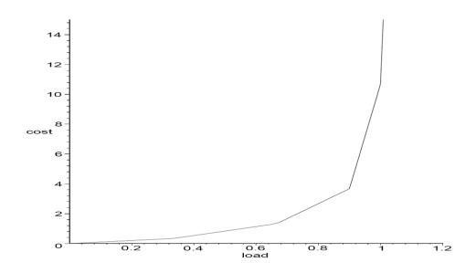
Figure 2.2.1: Link cost  $\phi_a(l(a))$  as a function of load l(a) on link *a* for link capacity c(a) = 1. (Source: [30])
