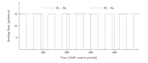
Figure 4.4.7: Two on-off traffic sources in Experiment 3.
