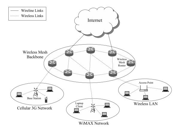
Figure 6.3.1: Example of an infrastructure/backbone wireless mesh network.
