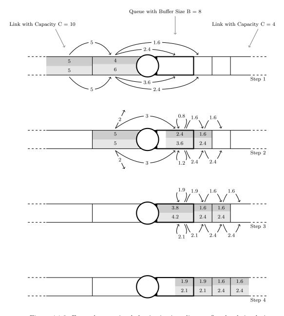
Figure 4.1.3: Example queueing behavior in time-discrete flow-level simulation.
