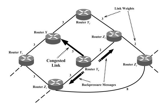
Figure 3.1.1: Basic idea of the backpressure mechanism.
