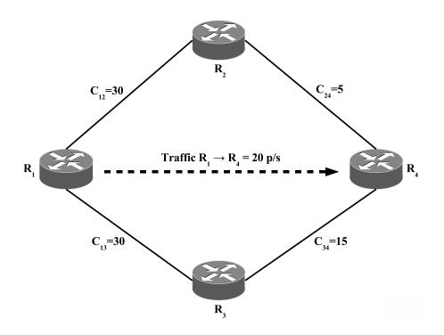
Figure 4.4.1: Setup of Stability Experiment 1 demonstrating AMP's convergence towards a stable traffic distribution.
