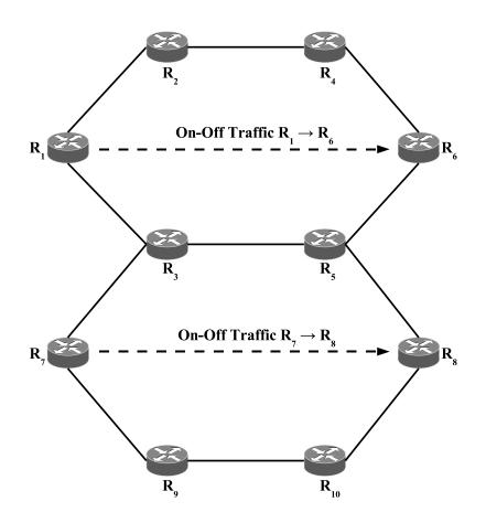
Figure 4.4.6: Setup of Stability Experiment 3 featuring two interferring on-off traffic streams.
