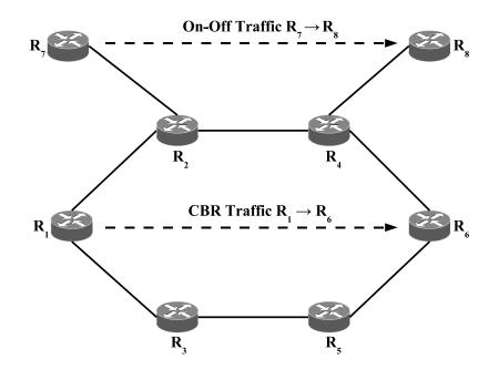
Figure 4.4.3: Setup of Stability Experiment 2 involving CBR and on-off traffic.
