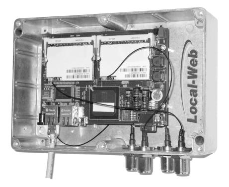
Figure 6.3.5: Local-Web wireless backbone router. (Source: [123])
