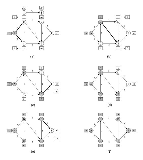
Figure 2.1.3: Illustration of Dijkstra's algorithm (extending Figure 4.7 from [19]).
