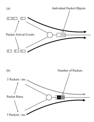
Figure 4.1.1: (a) Packet-level simulation vs. (b) flow-level simulation.
