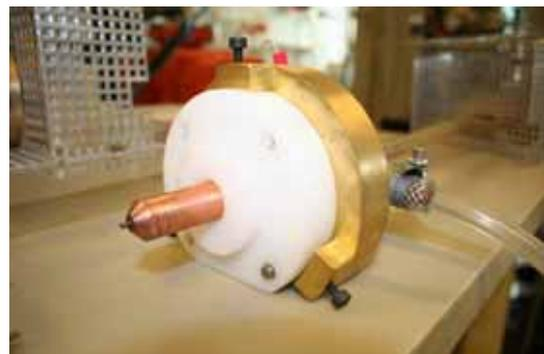
Figure B.4: Detail of the not moveable insulated water cooled cathode.
