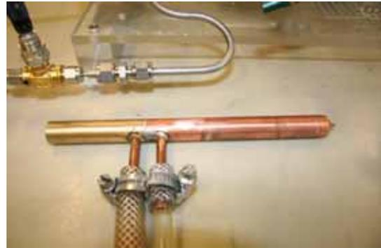
Figure B.2: Water cooled moveable anode.
