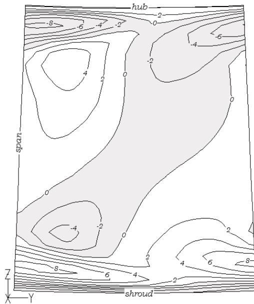
Figure 41 - Dimensionless vorticity of the cascade K_C .
