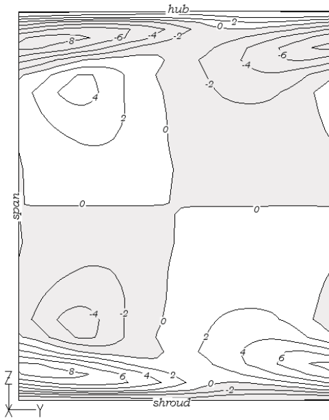
Figure 38 - Dimensionless vorticity of the linear cascade.
