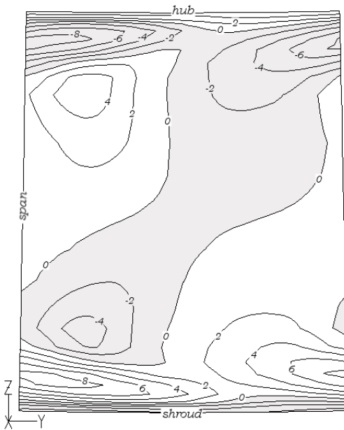
Figure 40 - Dimensionless vorticity of the cascade K_B .
