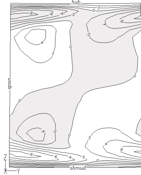
Figure 39 - Dimensionless vorticity of the cascade K_A .
