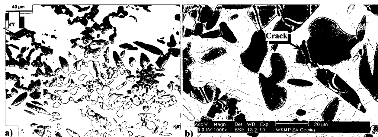
Figure 77. Ti662 reinforced with 12%TiC particles deformed up to \epsilon \sim 0.3 at 650^{\circ}C , strain rate 0.15s^{-1} a) and b) showing TiC-particle fracture
