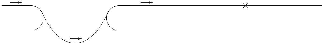
(a) A cable hanging between two 'tables' is drawn on the one end and pushed on the other end.
