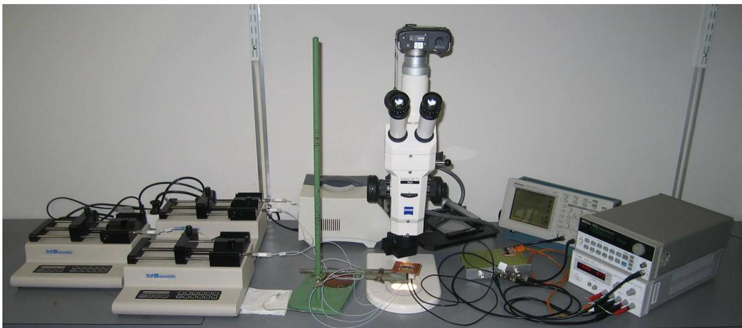
Figure 5.11: Photograph of the experimental setup. On the left are three syringe pumps placed, in the center can the stereo microscope and the device holder with the mounted PCB and device be seen and on the right are the amplifier, the power sources and the oscilloscope.
