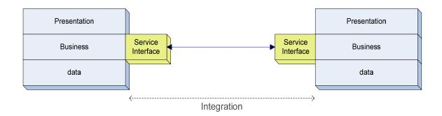
Figure 2-1 A logical representation of a service oriented architecture
