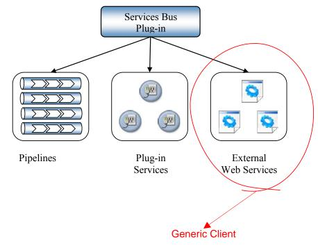
Figure 5-1 SOPA service Bus Plug-in and the location of generic client
