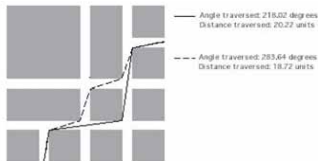
Figure 126: Minimum Euclidean path and minimum angular path
