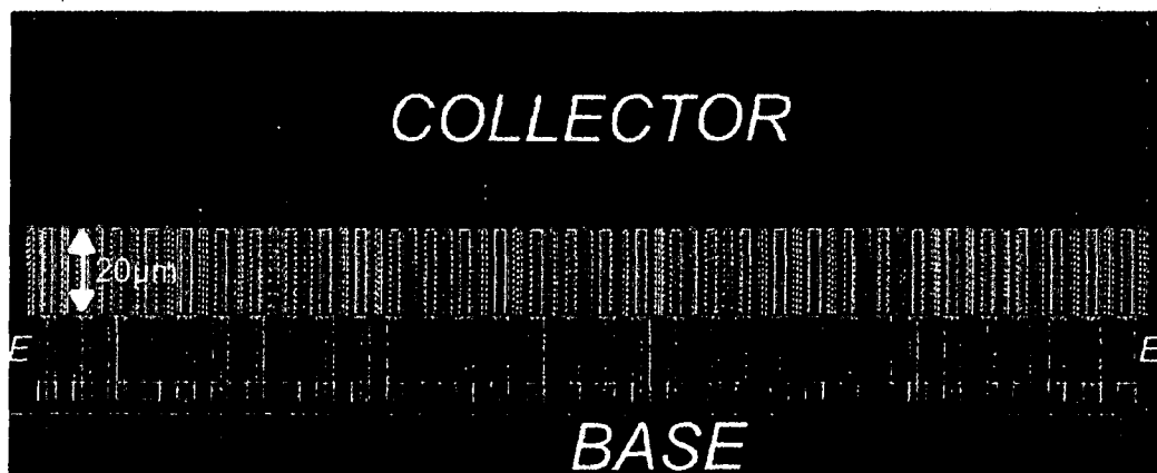
Figure 5.19: Layout of the output transistors T3 and T4. The 32 parallel-connected transistor cells features a double base, single emitter, double collector configuration. The emitter length is 20.4\ \mu\text{m} and the effective emitter width 0.5\ \mu\text{m} .
