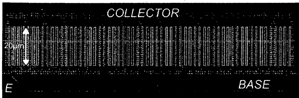
Figure 6.5: Layout of the output transistors T3 and T4. The 15 parallel connected transistor cells feature a triple base, double emitter, double collector configuration. The emitter length is 20.4 \mu\text{m} and the emitter width 0.75 \mu\text{m} .
