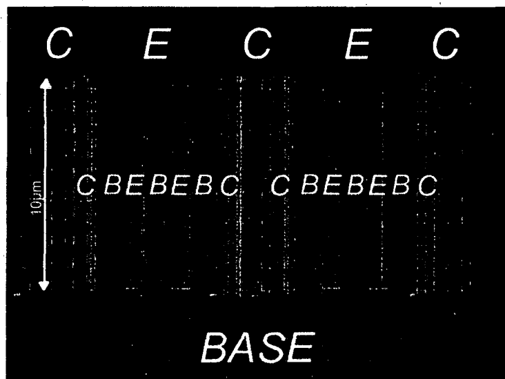
Figure 7.4: Layout of the driver stage transistors T1 and T2. The doubled transistor cell features a triple base, double emitter, double collector configuration. The emitter length is 10.2 \mu\text{m} and the effective emitter width 0.5 \mu\text{m} .
