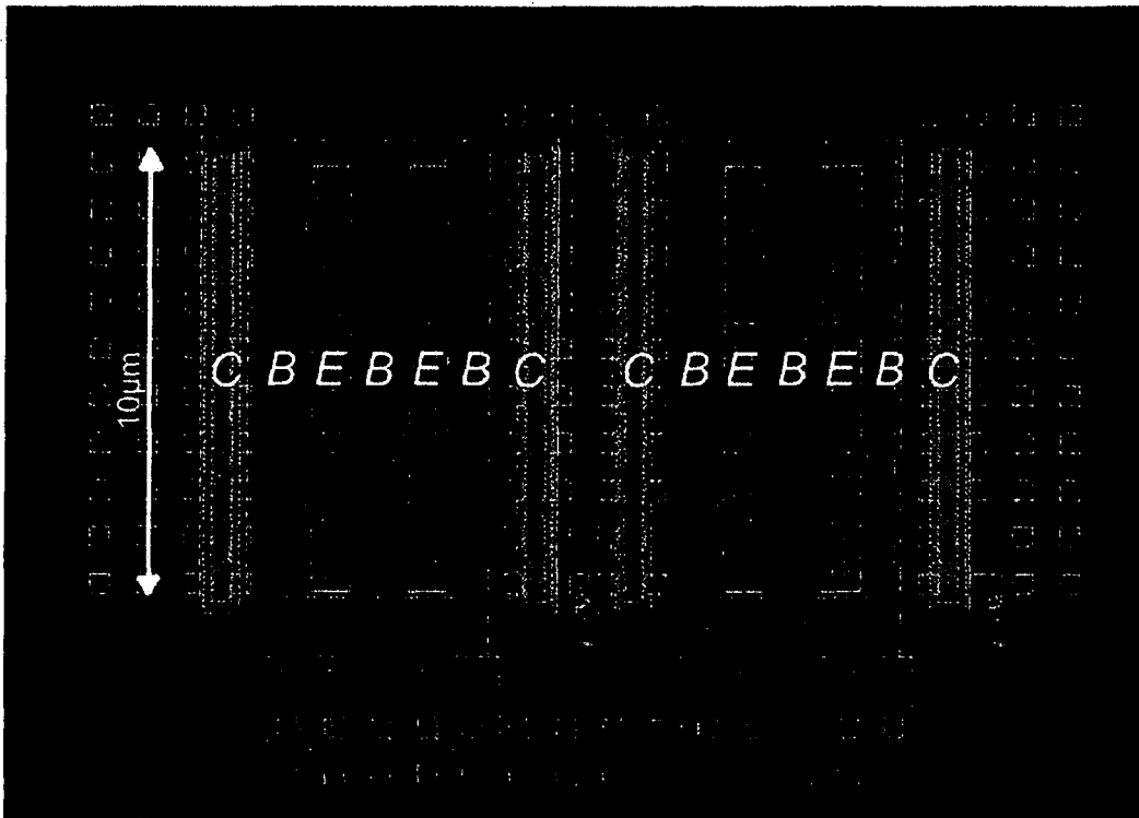
Figure 6.4: Layout of the driver transistors T1 and T2. The 2 parallel connected transistor cells feature a triple base, double emitter, double collector configuration. The emitter length is 10.2 \mu\text{m} and the emitter width 0.75 \mu\text{m} .
