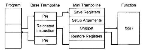
Fig. 5.2. The dynamic instrumentation control flow.
