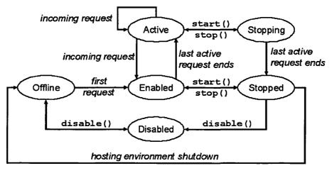
Fig. 5.7. The state transition diagram of the WASP-based Web services.
