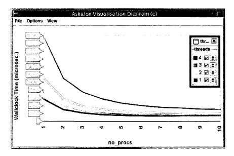
(a) Wallclock time for various intra-node and inter-node machine sizes.
