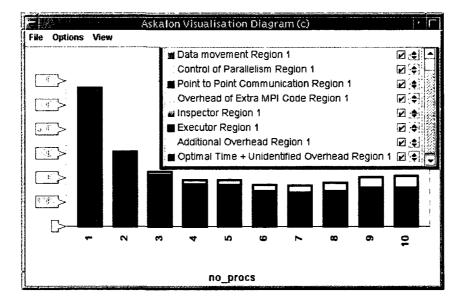
(b) Contribution of the MPI and the HPF overheads to the wallclock time, for various inter-node machine sizes, four threads per SMP node.
