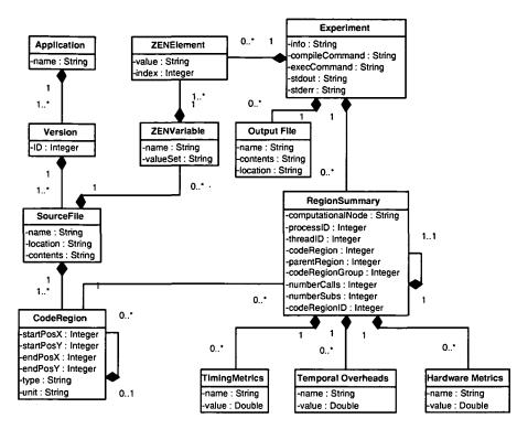
Fig. 4.9. The Experiment Data Repository schema definition.
