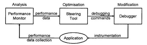
Fig. 5.14. The Steering configuration.
