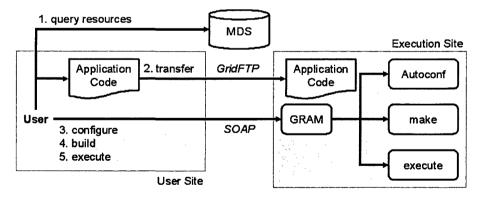
Fig. 2.8. Execution model of parallel applications on the Grid.
