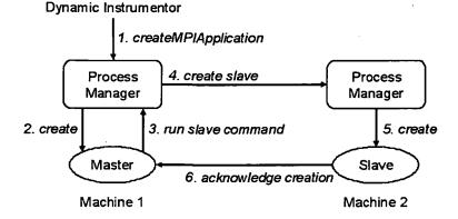
Fig. 5.5. Starting an MPI(CH) application for dynamic instrumentation.
