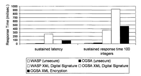
Fig. 5.17. Secure versus unsecure response time comparison.
