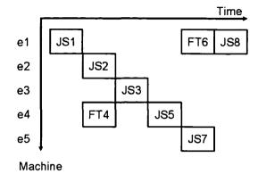
Fig. 6.5. Sample Gantt chart for the workflow depicted in Figure 6.4(b), assuming that  $e_2 = e_3$  (i.e.,  $S_{JS_2} = S_{JS_3}$ ).
