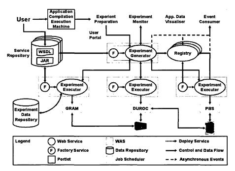
Fig. 4.1. The ZENTURIO experiment management tool architecture.
