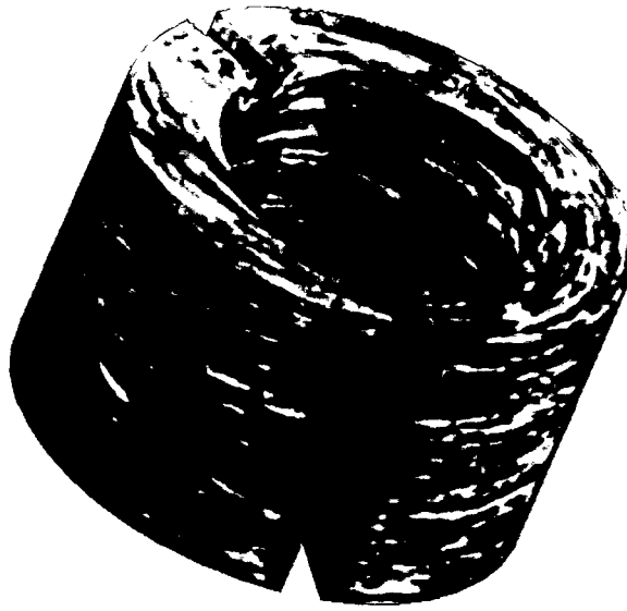
Figure 5.4: The result of applying a higher contrast normal mask to a ring data set. The texture is no longer visible at the inlet of the ring where the texture reflects the flow orthogonal to the surface. Compare with Figure 4.5 on page 52.
