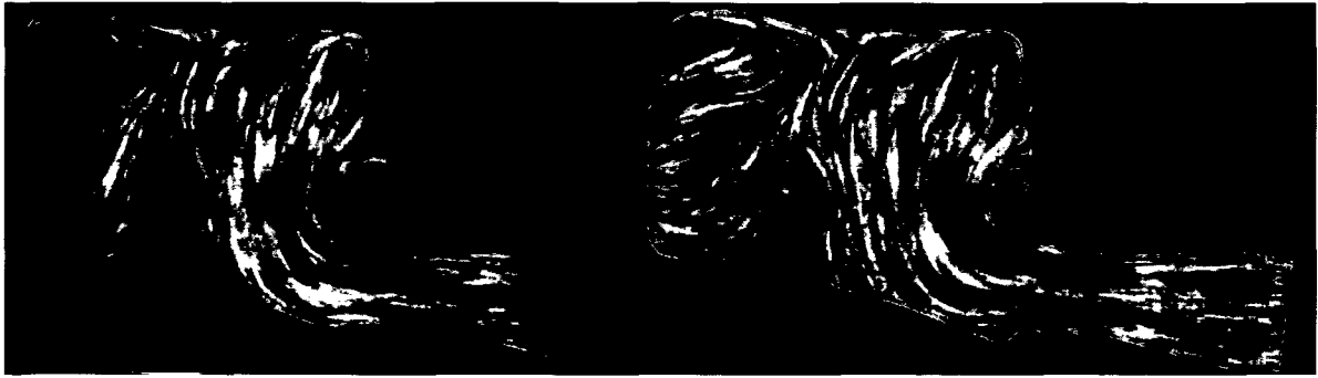
Figure 4.9: Here we see a 2D slice through a 3D geometry from a CFD simulation. (top) With no edge blending, the background color shows through boundary areas with incoming flow. (bottom). With edge blending, these artifacts are no longer a distraction.
