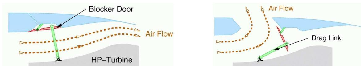
FIGURE 1.4: Operation of a blocker door. Flight position (left) and thrust reverser position after landing (right)
