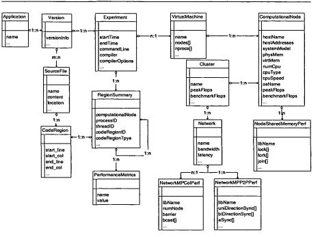
Fig. 5.3. SCALEA experiment-related data model
