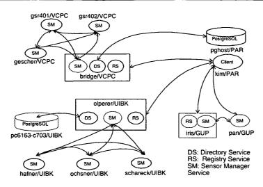
Fig. 7.26. Grid experimental test-bed.
