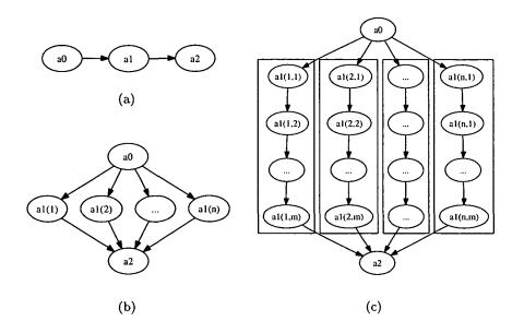
Fig. 6.22. Multiple workflows of an workflow-based application: (a) Sequence workflow, (b)Fork-join workflow, and (c) Fork-join structured block of activities.
