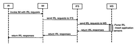
Fig. 6.17. Steps in conducting a request for instrumentation.
