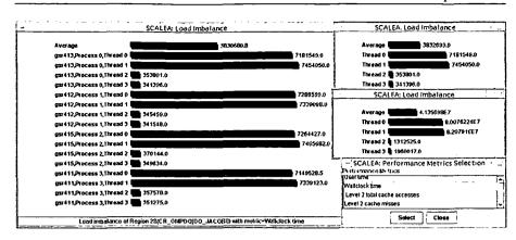
Fig. 7.4. Load imbalance analysis of an OMP DO code region in the subroutine  $DO_JACOBI$  executed with 4SMP nodes.
