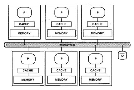
Fig. 3.2. MPP machine model.
