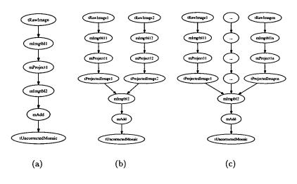
Fig. 7.33. Experimental workflows of the Montage application: (a) workflow executed on single resource, (b) workflow executed on two resources, and (c) workflow executed on n resources.
