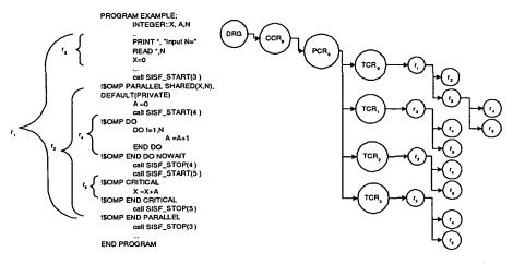
Fig. 3.11. OpenMP code excerpt with DRG when executing with 4 threads (denoted by  $TCR_0 - TCR_3$ ). Code regions  $r_1, r_2$  are executed only in thread 0 whereas  $r_3, r_4, r_5$  are executed in 4 threads. This program is running with 1 process (denoted by  $PCR_0$ ) on a computational node (denoted by  $CCR_0$ ).
