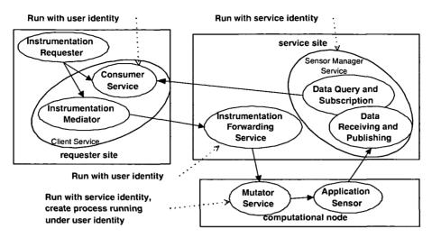
Fig. 6.16. Architecture of the Grid service of dynamic instrumentation
