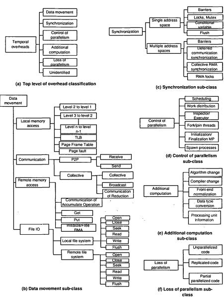
Fig. 5.1. The classification of temporal overhead.
