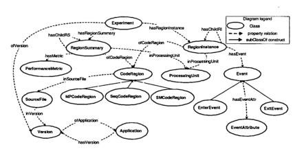
Fig. 6.24. Illustrative classes and properties of experiment-related concepts.
