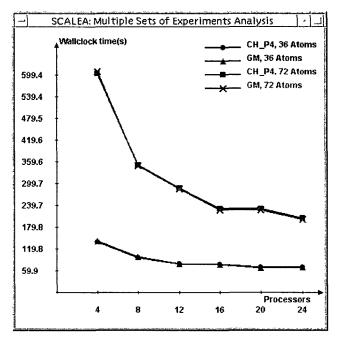
Fig. 7.20. Execution time of LAPW0 with 36 and 72 atoms. *CH\_P4, GM* means that MPICH 1.2.3 has been used for CH\_P4 (for Fast-Ethernet 100Mbps) and Myrinet, respectively.
