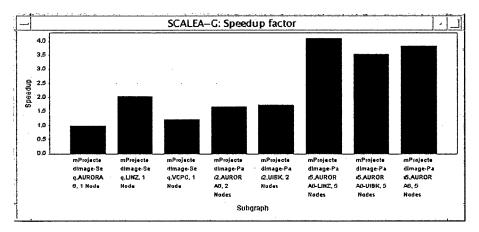
Fig. 7.39. Speedup factor for subgraph ProjectedImage of Montage workflows.
