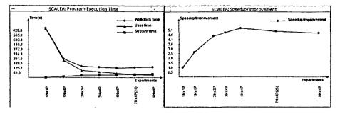
Fig. 7.15. Overall execution time and speedup/improvement for 3DPIC. 1Nx4P means 1 SMP node with 4 processors (in case of 7Nx4P only 25 processors are used)
