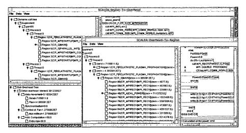
Fig. 7.12. Overhead-To-Region and Region-To-Overhead analysis
