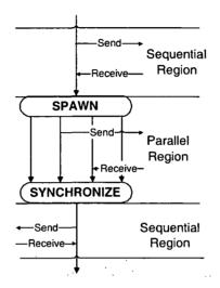
Fig. 3.5. Execution model of a single process in hybrid parallel program.
