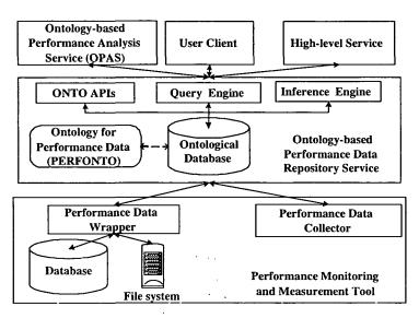
Fig. 6.27. Three layers architecture for ontology-based performance analysis, data sharing and tool integration
