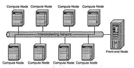
Fig. 3.3. Model of a cluster machine.
