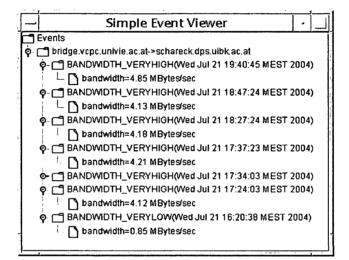
Fig. 7.31. Events generated from a rule-based sensor monitoring network bandwidth.
