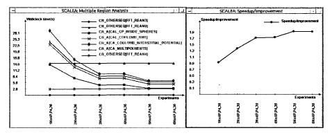
Fig. 7.21. Execution time of computationally intensive code regions. 1 Nx4P, P4, 36 means 1 SMP node with 4 processors using MPICH CH\_P4 and the problem size is 36 atoms.
