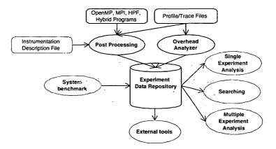
Fig. 5.4. Components interacting with the experiment data repository.
