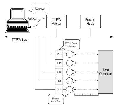
Figure 7.6: Setup for sensor fusion testing
