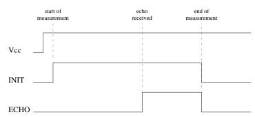
Figure 6.6: Timing diagram for the ultrasonic sensor
