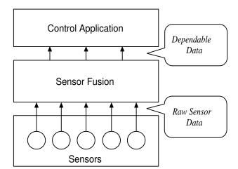
Figure 5.1: Sensor fusion layer converting redundant sensor information into dependable data
