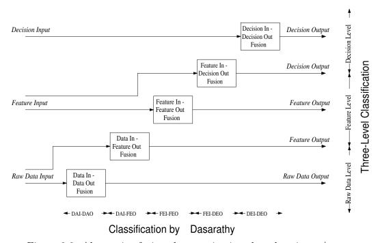
Figure 2.2: Alternative fusion characterizations based on input/output
