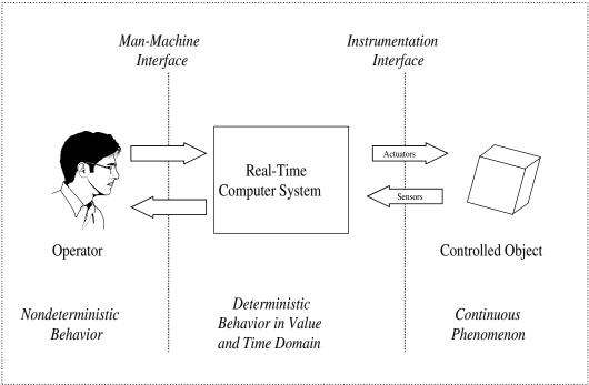
Figure 2.4: Parts of a real-time system
