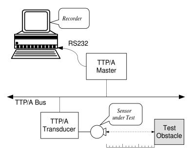
Figure 7.1: Setup for individual sensor testing
