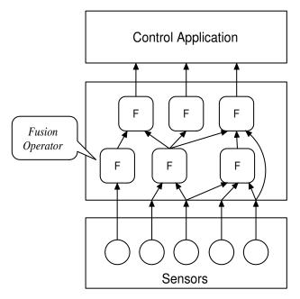
Figure 5.3: Structure of sensor fusion layer
