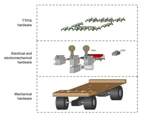
Figure 6.2: Hardware parts of smart car (from [Dia02])
