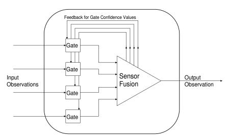
Figure 5.2: Structure of fusion operator
