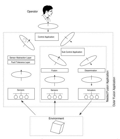
Figure 4.3: Nested configuration with intelligent control interface
