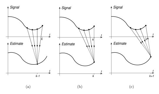
Figure 3.6: Smoothing (a), filtering (b), and prediction (c)
