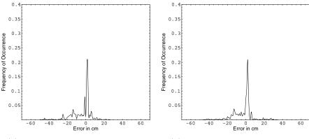
(a) Fault-tolerant sensor averaging
