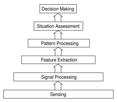
Figure 3.2: The waterfall fusion process model (from [Mar97b])
