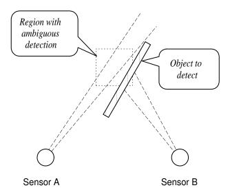
Figure 5.6: Discrepancy between sensor A and sensor B due to object shape
