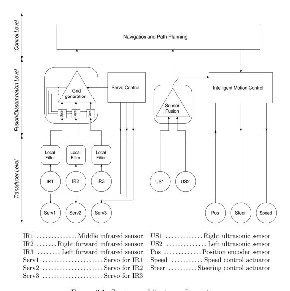
Figure 6.1: System architecture of smart car
