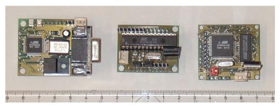
Figure 6.7: Employed TTP/A node types (from left to right: master node with monitoring interface, slave node based on AT90S4433 MCU, slave node based on ATMega128 MCU with external RAM; scale in centimeters)
