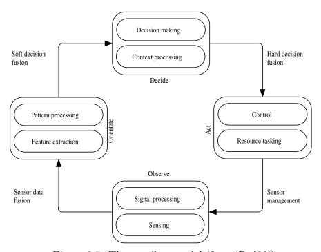
Figure 3.5: The omnibus model (from [Bed99])
