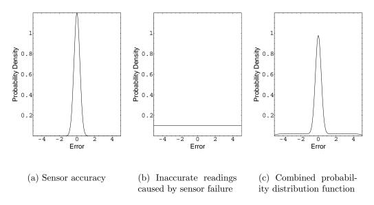
Figure 5.4: Example for sensor behavior regarding accuracy and failure
