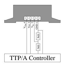
Figure 6.5: Connection diagram for the GP2D02 infrared sensor
