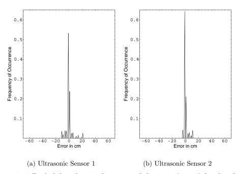
Figure 7.4: Probability density functions of the error (in cm) for the ultrasonic sensors
