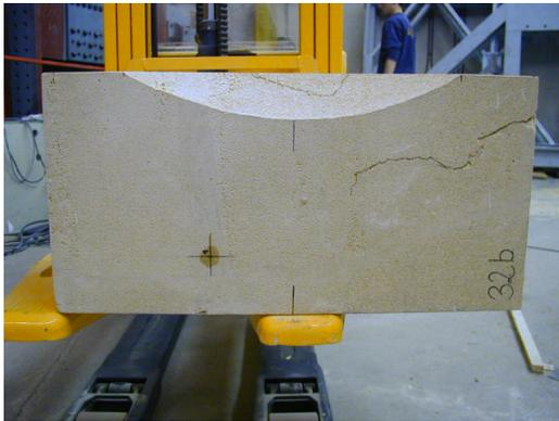
(c) Fractured specimen 32b side view, fracture pattern A
