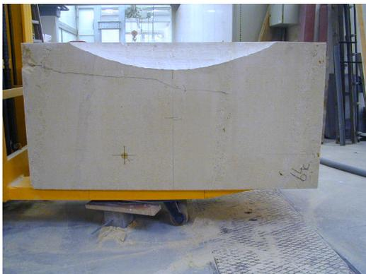
(e) Fractured specimen 64c side view, fracture pattern B
