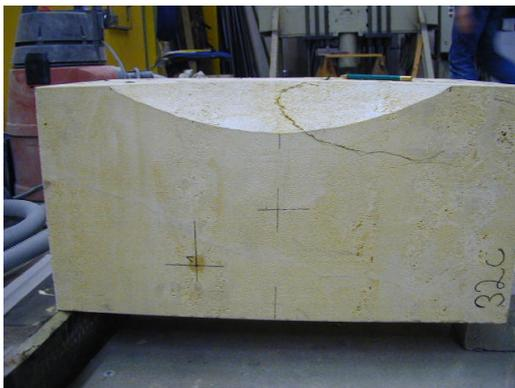
(e) Fractured specimen 32c side view, fracture pattern A
