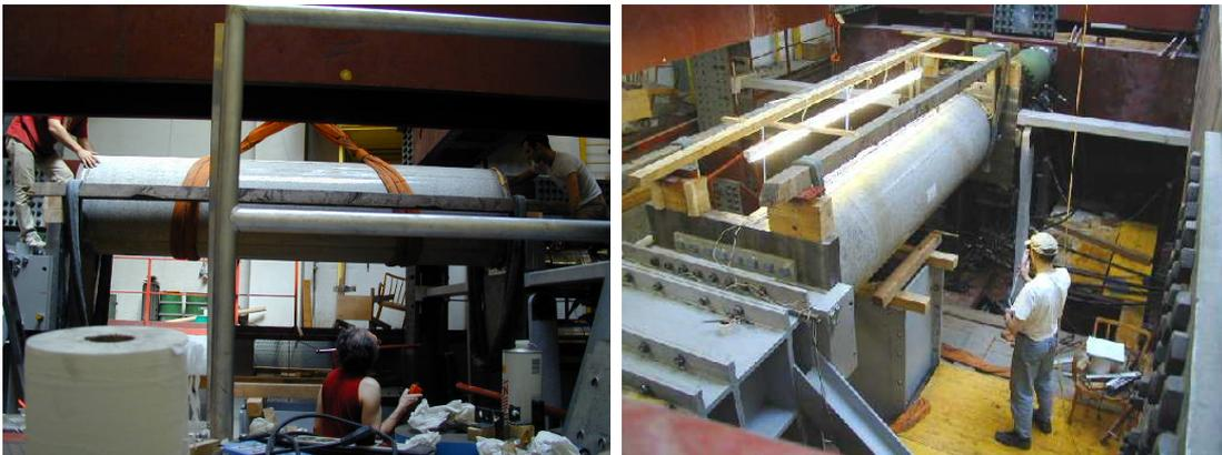
Figure 8.9: Installing of specimen 80b in the Column Tester (left). Specimen 80 b prior to testing (right)
