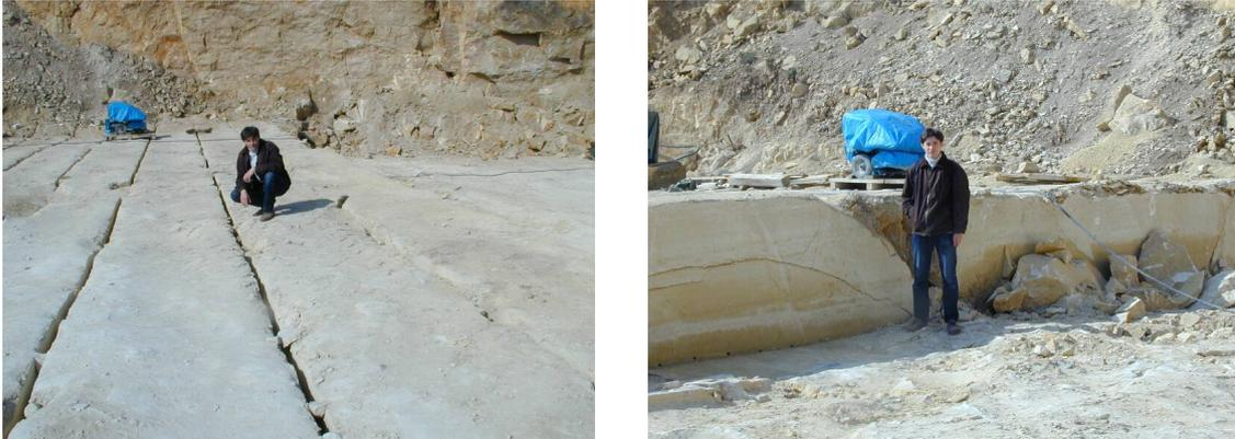
Figure 3.1: Sandstone in the quarry "Hummel". Left: Vertical cuts after sawing. Right: block of sandstone
