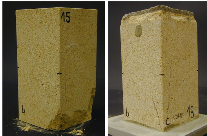
Figure 4.4: Spalling of edges when tested directly on steel plates (left) and when fine grout layer was used (right)
