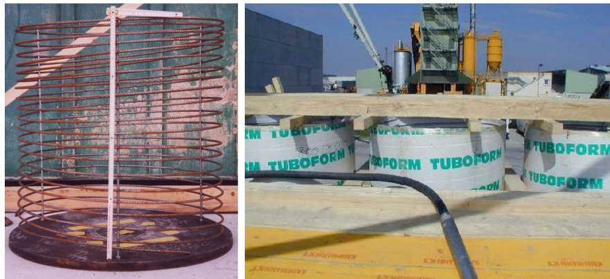
Figure 8.5: Reinforcement which was inserted at bottom of the specimen(left). The construction for fixing the reinforcement at the top of the specimen and at the same time for fixing the cardboard tube in vertical direction (right)
