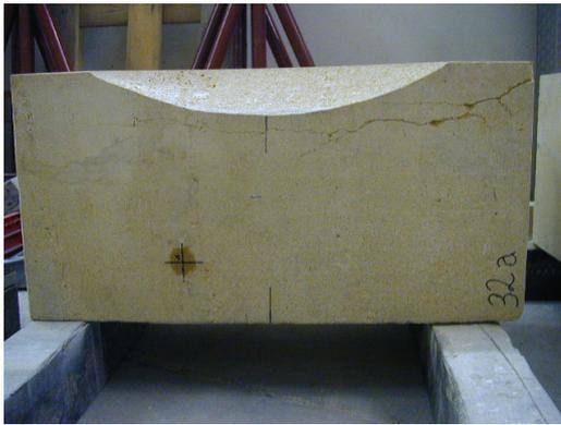
(a) Fractured specimen 32a side view, fracture pattern B
