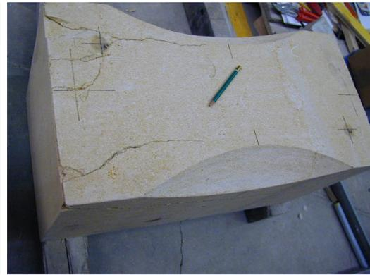
(b) Fractured specimen 32a top view, fracture pattern B
