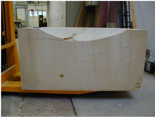
(a) Fractured specimen 64a side view, fracture pattern A
