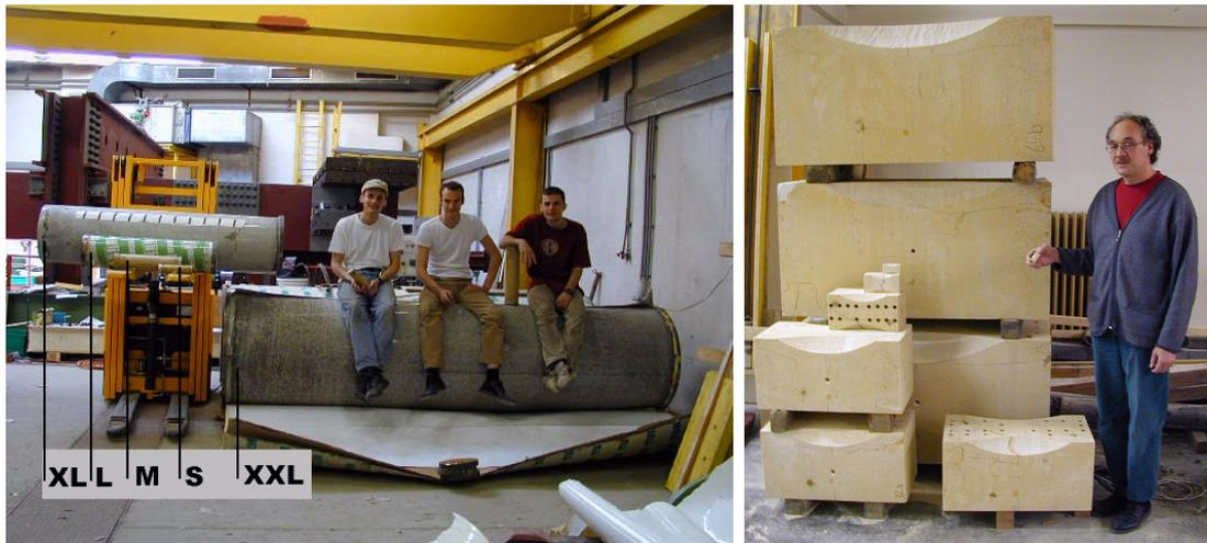
(a) Specimen of concrete series on sizes S (diameter 5cm) to XXL (diameter 80cm) (b) Specimen of test series on sizes XS to XXL (smallest specimen in hand)
