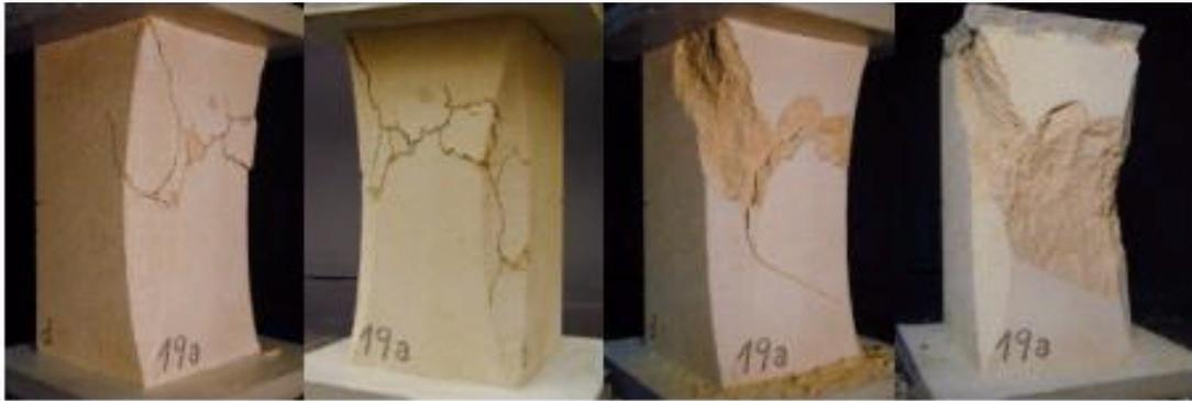
Figure 4.14: Specimen 19 after testing and opening the existing cracks (from left to right)
