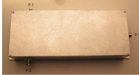
Figure 4.38: Bias-T for Pulses up to 100 \mu s
