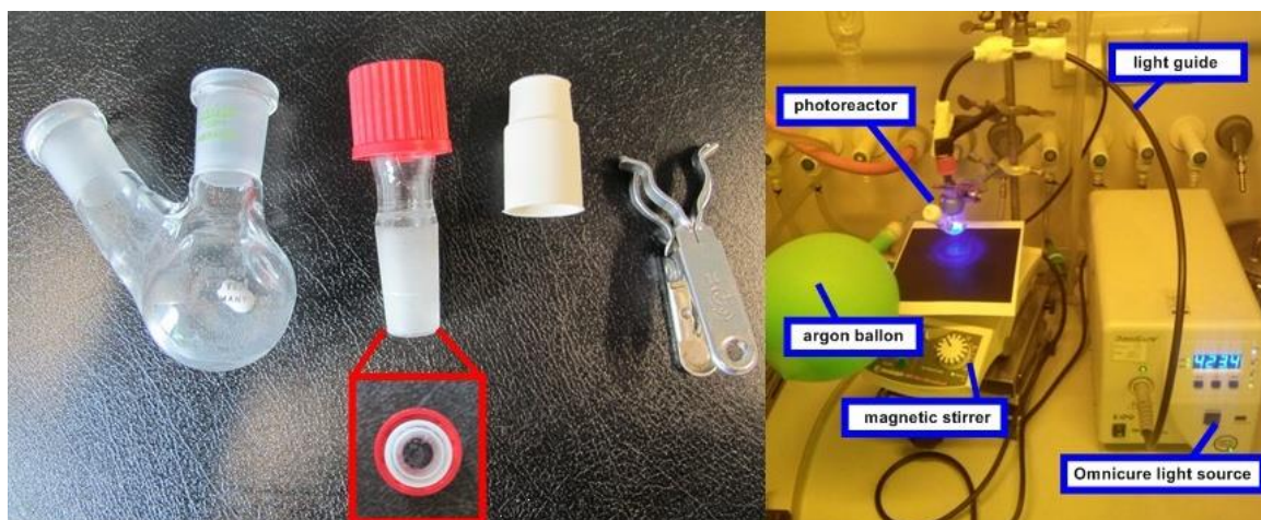
Figure 126: Typical photoreactor setup
