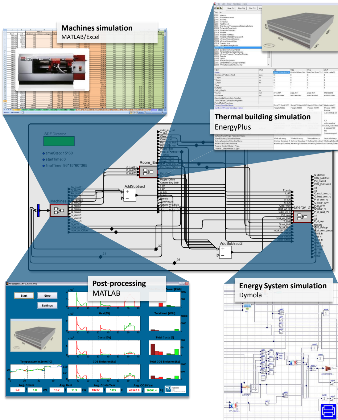
Figure 2.12: Overall co-simulation framework instance for the case study with BCVTB middleware as well as MATLAB, Dymola and EnergyPlus simulation clients and post-processing in MATLAB.
