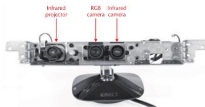
Figure 3: Components of Microsoft Kinect™ sensor v1 (reprinted from (Zhang, 2012))
