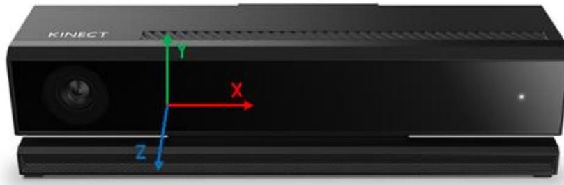
Figure 7: The camera space coordinate system (adapted from (Microsoft, 2016a))
