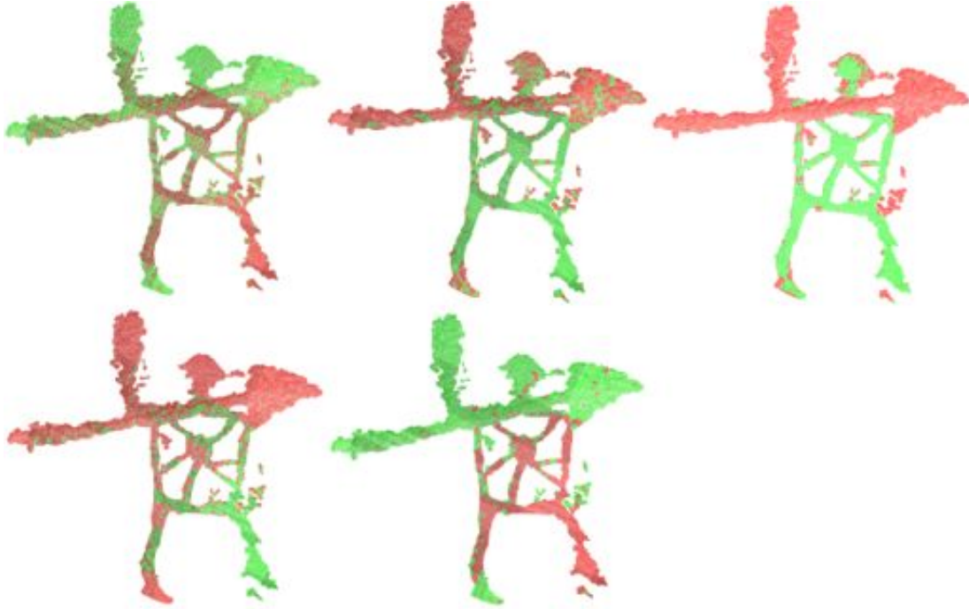
Figure 6.10: Comparison of different descriptors and footprints. The first row shows clustering results based on the FPFH descriptor with r=1, 2 and 5\text{mm} (from left to right). The second row contains clustering with PFH with r=1 and 2\text{mm} (from left to right). We observe, that this scan requires a large descriptor footprint as the best result is FPFH with r=5\text{mm} . The original scan is shown in Figure 6.2.
