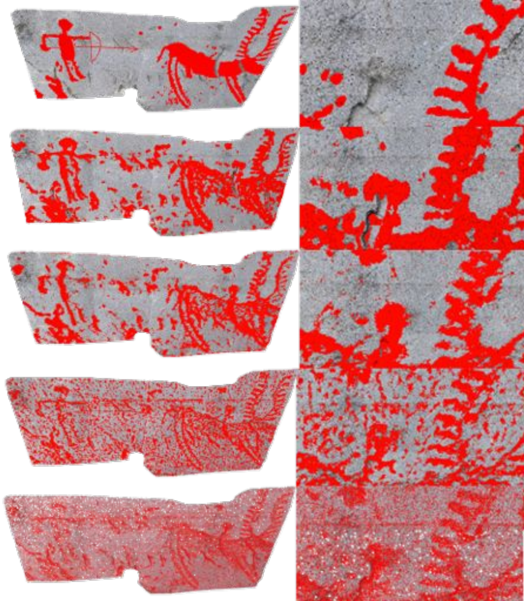
Figure 5.3: Qualitative evaluation of the discriminative abilities of the employed 3D point cloud geometry-based descriptors. The rows from top to bottom show the ground truth, PFH, FPFH, SHOT and 3DSC. The right hand side shows details. We observe, that each point cloud descriptor produces a large amount of false positives compared to the ground truth in row 1.
