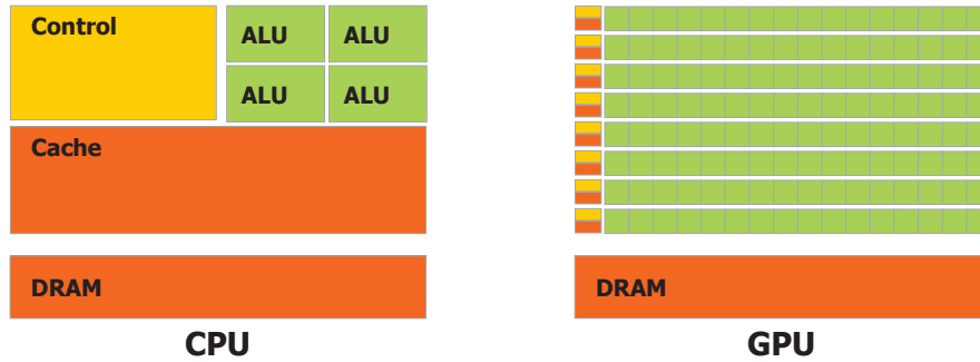
Figure 5.2: Comparison of CPU and GPU architecture: the GPU devotes more transistors to data processing.
